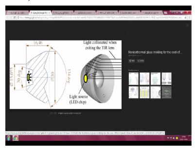
In case you have a chip LED, you now end up with having to design things which are a little like this. So we have the lens here. That lens will also ensure that the light can get collimated. This data from here we probably need to build up in all of our things as we move along. Now coming back to the, my other monitor, the, what you call, drawing I am making. You please look at the other monitor.
