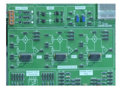
So now we have covered the power section of the board, the DC-DC converter section of the board, the diodes in the board trimmers. And then we looked at the op amp inverting how the inverting op amp a functions then and can be tested.
