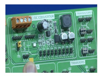
So, this is how a jumper looks like this yellow jumper. So, how does jumper look like? So, inside one end are holes see here. These holes so, they will have 2 pins, 2 insert locations and then at the top these pins will be connected. So, these are connected here shorted. You will be able to see here. So, if you can check with same jumper is connected here. So, here see at top there is a metal piece. So, that will connect this berg to this berg.
