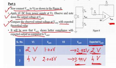
So, I have a gain of 2, right; that means, if i apply 2 volts if my expected output would be expected output should be 2 volts across R 1 and R 2. So, this is 1 volt, 1 volt by gain of 2 1 volt into 2, so output will be 2 volts right.
