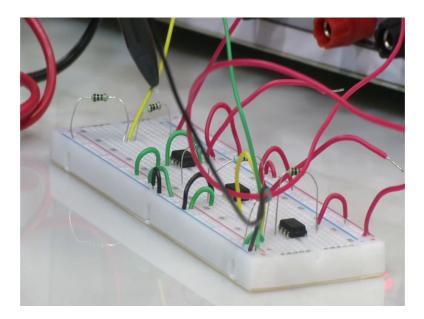
This is a potential divider circuit which is this one and we have applied 2 volts across it. This is a potential divider circuit, we are applied to volts and then yellow colour wire is the output is output is a voltage across resistor R 2 alright. So, let us see what is the value of resistor R 2, voltage across R 2. Voltage across R 2 is 1.009 volts, voltage across R 2 is 1.009 volts.
