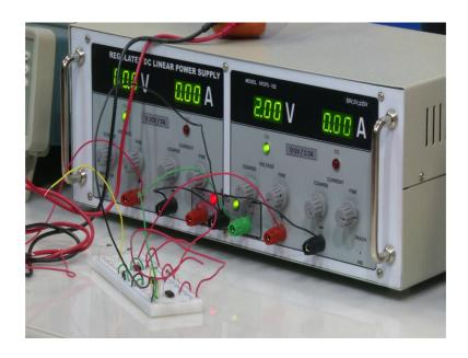
Across the potential divider circuit, he is applying 2 volts. As you can see on the DC power supply, you can see 2 volts, which is given to the potential divider circuit which is same like last time if you remember right.
