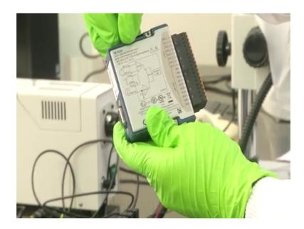
And this is another one, which I already told you. It is analogue input either voltage as well as current can be taken as an input to the system.
