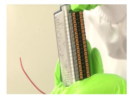
So, it has both positive terminal and negative terminal, what it does is that it can measure a differential input. Some cases where when you are using a quarter bridge or when you are using a half bridge or full bridge, whatever the voltage signal it is being generated from the bridge signals are not a independent voltage, it is a differential output voltage.
