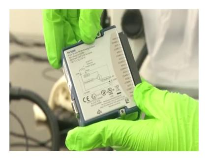
So, we also have analogue output, say it can produce up to 20 milliamps of current and it is a 16 bit analogue output too.
