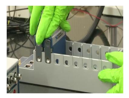
So, the advantage is that, it can be interchange, it need not to be fix only to the particular channel, even it can be fixed to the last channel anywhere wherever where it is required.
