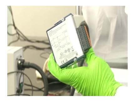
And other one is a quarter bridge analog unit. The difference between the previous module which I showed to this modulus is by making use of the previous model, you can perform a quarter bridge, half bridge and a full bridge, but by using this module we cannot perform half bridge as well as you know full bridge. This is only meant for quarter bridge applications.
