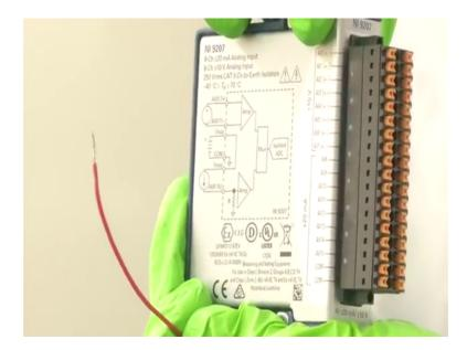
So, the first channel, so here if you see there is different number of channels starting from 0 to 7. So, total it has 8 channels for analogue acquisition which can measure up to plus or minus 10 volts.
