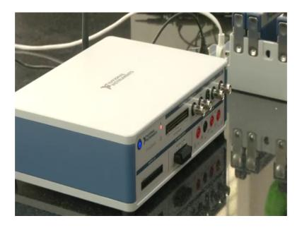
So, what I do is that, I will take few wires by using this work virtual bench, I will connect it to the DC power supply and if I vary the signal from the DC power supply, we can observe the signals being acquired using this CDAQ in our monitor.
