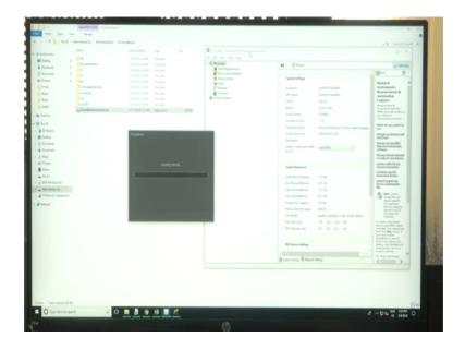
Start NI MAX. This is for CDAQ just to test the device has been connected and whether it is working or not.
