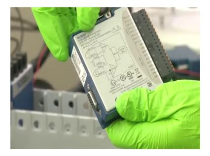
So, we can see here, 1 is analogue input channel, so where it can be used for input current as well as input voltage tool. And it has a on board ADC's as well as amplifiers everything.
