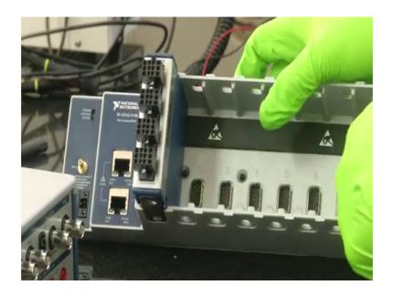
So, how to place in this in the sense, so if you see to the chassis, it contains different number of channels, so simply select the required signal conditioning unit or they call it as a module and place it on the appropriate channel.
