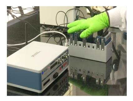
So, signals can be generated using PC from the virtual bench and the same signals can be acquired using another compact DAQ and can be acquired into this data acquisition device to the PC using this data acquisition device and even that we can visualise in between there is another software called lab view.
