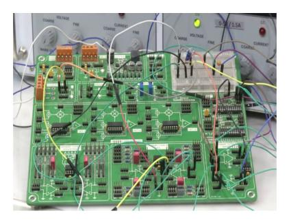
So, the circuit that we have described that is what we were what we just went through, digitally controlled square and triangular, triangular wave and square wave generator. So, what is the control here digitally, actually when you see the working of circuit, you will
