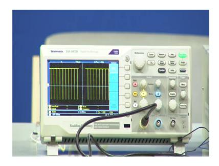
Now, let us see the output. So, you can see square wave here with the different duty cycle, it is not 50 percent duty cycle. So, we can see it clearly, square wave getting formed correct. So, we are seeing a nice square wave getting formed with a skewed duty cycle correct.
