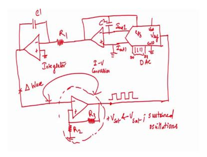
So, what all will be there again, first we will have you can draw it along with me, we can you can build the circuit along with me in your notebooks. So, first you will have the DAC system, correct first thing is first. The DAC system will have reference voltage, supply voltage, ground, which can you can ground automatically. Feedback path feedback resistor, I out 1, and I out 2, clear.
