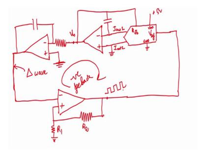
So, what we have to do, the triangular wave is there. So, now we will take it, and give it to the negative terminal of an op-amp. And output will be there, we have to give positive feedback, because it is a Schmitt trigger. I will say this is R 1, R 2. Now, the output of this Schmitt trigger, so here we will be able to see the square wave ok.
