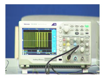
So, now this is a different frequency correct, it is coming a nice duty cycle square wave, correct. So, let us change another bit now. So, see you can see that the frequency has changed correct with the different duty cycle. So, if we change another bit, again the frequency will change see, the frequency has changed drastically now, you can see it correct. So, this way we are able to digitally program the frequencies, for the triangular and the square wave using the DAC module.
