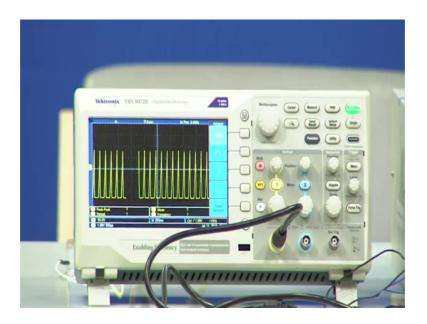
So, we are seeing the oscilloscope correct. So, you can see nice triangular wave getting formed of a particular frequency, correct. Now, let us just see the oscilloscope only. Now, I will remove that yellow wire for the signal, take it from there, and connect it to the output of the Schmitt trigger to see the square wave ok.
