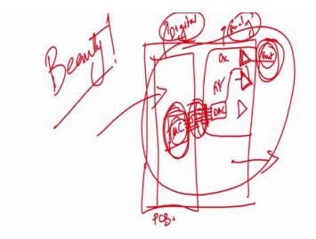
So, let suppose we have a PCB and you have an analog analogue section in the PCB and you have a digital section clear. And your digital section is controlled by say a microcontroller mu C you have with the analog domain which have lot of amplifiers. Let us say and other filtering filters and all source of oscillators filters everything oscillators filters all these are analog domain this is your analog domain this is your digital domain of the PCB ok.
