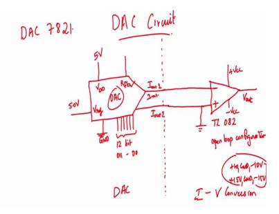
So, this much portion is your digital to analog conversion correct now we have the current to voltage conversion correct. So, what to do for to do that what do you need so you need to connect an first you put a op-amp.
