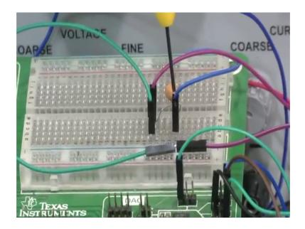
This capacitor we have connected between the feedback line and the inverting input terminal as per the circuit design for avoiding gain peaking ok. Now, we are all set to see the connections now let us focus on the tri state logic for the bit sequence ok, now you can see it. So, if you see now we what we will do is we have given supply everything is then ready.
