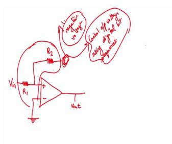
Here is where so here there should be something that can do two things what all one is give a negative output negative voltage negative voltage contribution another is controlled output voltage using digital bit sequences correct two things you should have negative voltage. So, that we will have negative feedback so the amplifier operation can work properly and we should have controlled output voltage that will change with bit sequences.
