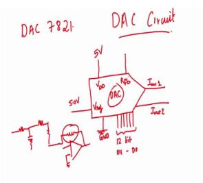
So, how it will DAC be so after seeing the datasheet I showed you what are the important signals that you need to look at right. So, let us just show the DAC like this the DAC is shown. So, what are the main things first is ground anywhere for any IC you will have ground so ground will be there clear then what else supply will be there. So, VDD then because it is a digital to analog converter it will have a reference voltage also it is called Vref ok.
