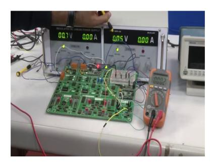
The input voltage is applied from this power supply there plus 15 minus 15 supply for the op-amps is given from this power supply the central power supply. So, we are applying an input of 0.05 volt or 50 milivolt and that that signal is applied to this; and through the resistor here. So, that signal is applied through the resistor here then now we will see the output by looking at the output of the op-amp.
