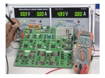
Because we have use the inverting configuration we will get negative voltage as a output. Let us now focus on the multimeter: yes, now we can you can clearly see it correct. So, what we are saying so our bit sequence is 0 0 0 0 0 0 last bit 1 so we have got 28.5 millivolt correct around 28.5 millivolt.
