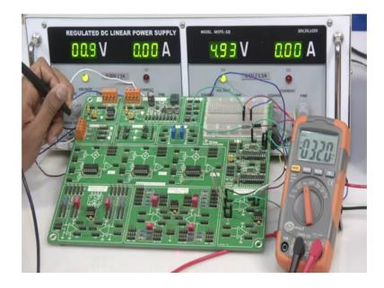
That is  $D \ 0 \ D \ 1$  are one now instead of keeping  $D \ 0 \ D \ 1$  as 0 and then changing  $D \ 2 \ D \ 1$  we will do  $D \ 0$  high  $D \ 1$  high  $D \ 2$  high. So, instead of getting 1.5 to 2 millivolt increase per bit change we will get double of that around 4.5 to 5 here we are getting around 5.5 millivolt, but roughly in that range we will get.
