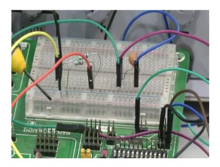
So, here we have connected the two resistors as we have seen so we have seen right. The amplifier in which the input was connected to the positive terminal of the op-amp through a resistor and the feedback path had a resistor on it that is connected to the DAC at digital to analog converter system.
