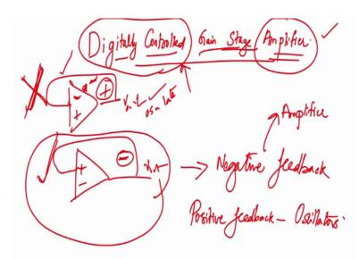
Fraction of the positive voltage of your output to your negative terminal correct this is negative terminal correct. Or how you can do negative feedback you can convert a portion a negative portion of your output voltage to your positive reference that is also negative feedback correct is the two ways you can do it.
