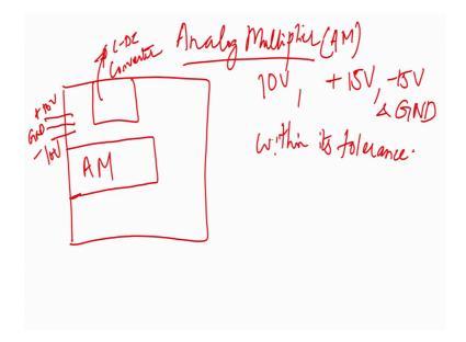
So, we are basically trying to understand the analog multiplier how they work? So, if you remember the board. So, you had the board you had the DC DC converter section here, and you had the analog multiplier section here. Let us call analog multiplier AM here for quick reference. Now the board had input of as per expectation the boards inputs where suppose to be plus 10 volt, minus 10 volt and ground correct.
