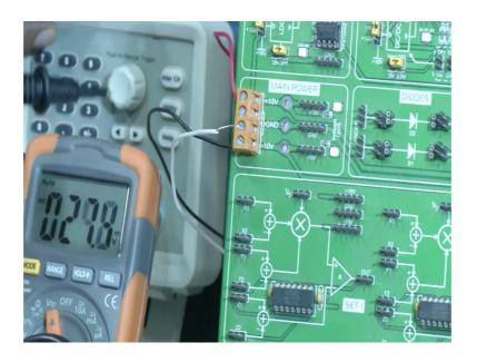
So, the power LEDs are on that shows that the power is coming. So, we will just check what is the input voltage? So, as you can see in the multi meter here it is 15 volt, so input is there. So, now let us go back to DC DC stage. Yes we are in the DC DC stage.
