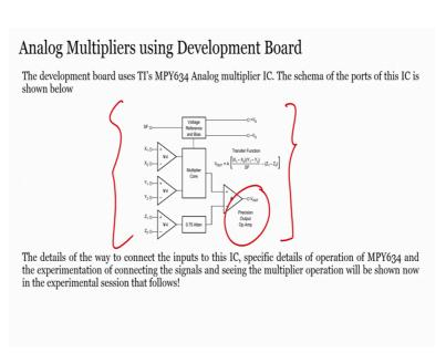
So, if I use at TI board and I want to design multiplier circuit. Then in the TI board we have MPY634 analog multiplier I C. And the schematic of the ports for this I C are shown in right over here right.
