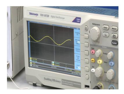
So, as you can see it as almost finished the sweep. So, it is like a 25 seconds sweep correct. So, if you look at it one sin wave one whole sin wave has taken how much? So, it has taken around half of the entire display area, so that is around 25 seconds correct.
