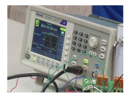
So, this is the function generator. So, as you can see we are using a sin sinusoidal signal of 1 kilo hertz frequency ok. So, that we will be giving and now let us look at the power supply DC DC here ok. So, we have given so behind your board can see the power supply power supply here.
