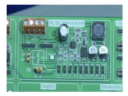
So, so this is the input voltage section like what is the input voltage you want to give. So, if you want to give an external different voltage you have this is a selection jumper selection pin, these 3 pin are the jumper selections. So, if you want to select from the board only then you have to use a jumper between these two pins bottom two pins.
