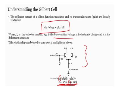
The collector current of a silicon junction transistor and it is transconductance are linearly related as you shown here right, where you can see that the collector current and the voltage between the base and emitter. If you take a division of that would be equal to q I C by k T and where I C is your collected current and V B E is a base emitter voltage, q is of course a electronic charge and k is a Boltzmann constant.
