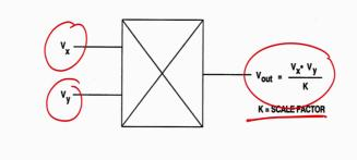
So, if you see the slide the basics of analog multipliers; when we say basics what does it have? Analog multiplier is a circuit fundamentally having two input ports and an output port. We are multiplying two signals let sus say V X and V Y and we get output as V X into V Y divided by K, where K can be a scale factor. So, in a very simple terms if you see an analog multiplier we can say having two input ports and one output port.
