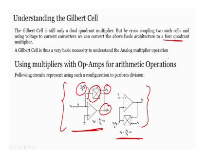
So, if you use current instead of voltages then the point can be solved. The limitations of the earlier circuit can be overcome. So, the Gilbert cell is still only a dual quadrant a multiplier as we can (Refer Time: 08:24) it is only dual quadrant, but if I want to make four quadrant multiplier what can I do?
