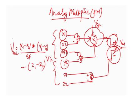
So, if you remember analog multiplier. So, there was 3 sets of inputs X 1, X 2, Y 1, Y 2, Z 1 and Z 2. Essentially there was a adder here and this was getting added plus and this was getting subtracted. Similarly and then this output was going to the multiplier and there was Y 1 again there was a adder here, plus was there, minus was there.
