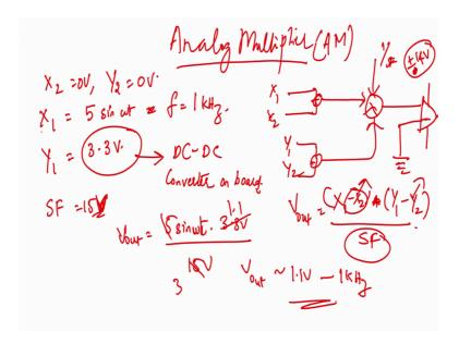
So, basically without looking an op amp wise what will be our function of scheme of operation? X 1 minus X 2 will be there and Y 1 minus Y 2 will be there. These two will go to a multiplier and they will get multiplied with a scale factor. And we get the output and this negative terminal would be grounded.
