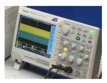
So, you can see the oscilloscope correct. So, as you can see we have stopped it. So this run and stop is kept because the output is having a very low frequency remember it is a frequency multiplier correct. So, the output is still sinusoidal and the peak to peak also got multiplied with the 3.3 volt ok.
