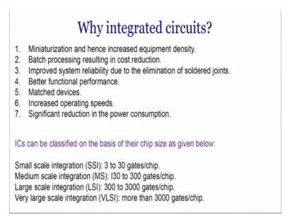
Then we talked about why integrated circuits and we could easily see why. there are several reasons: including miniaturization, batch processing, better function performance, matched devices, increased operating speed, and significant reduction in the power consumption, right. These are all the reasons enough reasons to make sure that we have to use IC instead of discrete components. And then we have also seen that ICs can be classified into several categories.
