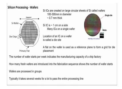
So, we will see that we have seen silicon wafer processing. So, silicon when you talk about processing of silicon and in terms of wafer on wafer. Then we have individual chips at the end of the fabrication process and each chip is called a die right each chip is called a die. And then we also seen that there is a primary flat, and this primary flat is for a purpose what is the purpose of primary flat to understand with respect to secondary flat.
