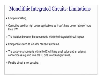
Then we have seen that what are the limitations and the limitations are lower power rating isolation between components within the integrated circuit is poor components such as inductor cannot be fabricated the passive components within the IC have small value and if you require IC passive components of higher values.
