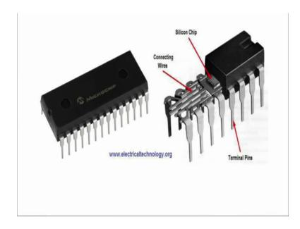
So, after this we moved to op-amps and silicon chip when we see the silicon chip, right this is this entire IC can be an operation operational amplifier.
