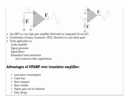
Then we saw; what are the advantages of op-amps over transistor amplifier. So, there are several advantages that are listed over here right which are less power consumption, it cost less.
