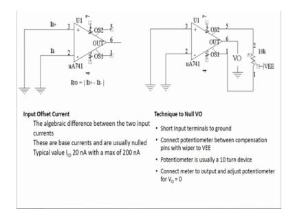
Input offset current right the algebraic difference. So, what is the technique to null the output voltage technique to null the output voltage you see when we short the input terminals 2 and 3 to ground, right. Practically should be 0 output voltage will be 0, right so, but it is not 0. So, we have to make it 0 that is called nulling output voltage.
