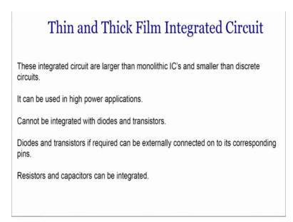
That is why we have to opt for thick and thin film integrated circuits. And here, the advantage is that the resistors and capacitors can be integrated cannot be integrated, it can be used in high power applications, while some limitations are it cannot be integrated with diodes and transistors, while if you want to use diodes and transistor, it can be connected externally on its corresponding pins.
