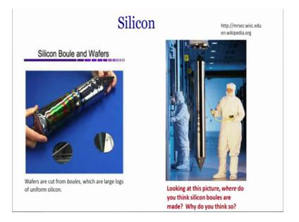
Then about the silicon right silicon is manufactured in a clean room in a clean room, what you can see in the right side is a Boule of silicon, right. And wafers are cut from this and polished to form the final wafers silicon is cut from this particular Boule to form final wafers, right.
