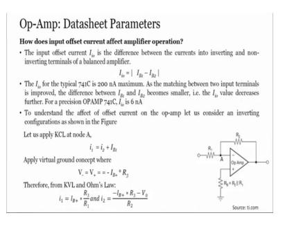
So, when you see input offset current input bias current input offset voltage you know CMRR, these are all datasheet parameters. So, just look at it thermal drift, right.
