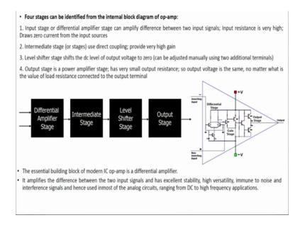
Then we have seen the internal stages of operational amplifier it consists of differential amplifier intermediate state level shifter, state output state. And most of the op-amps are now replaced by MOSFETs internal circuit that you see here BJT most of the cases. Now we are using MOSFETs, alright.
