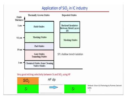
So, then we have also seen that for a for fabricating any sensor including MOSFETs, right, we need oxides, it can be gate oxide, it can be field oxide, it can be masking oxide and based on what kind of application of the oxide, we are using or based on the
