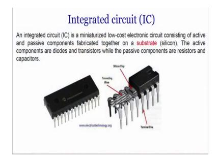
So, if you see, we talked about integrated circuit, and integrated circuit is nothing but miniaturized low cost electronic circuit consisting of active and passive components and it is built on substrate which is silicon. So, when you when you see a IC when you open an IC, you will see a silicon chip within the integrated circuit.
