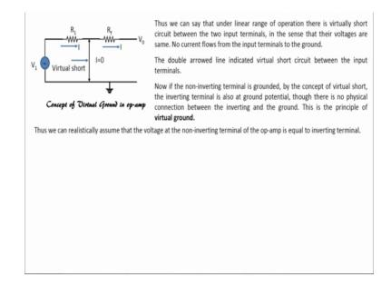
So, let us move forward we have seen the concept of virtual ground, right. So, even if one of the terminal is grounded the second terminal is also considered as a ground. And that is a concept of virtual ground.
