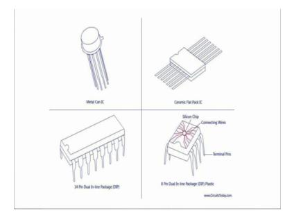
ICs when you look at the IC, it has metal can IC; that the ICs can be divided into few further categories metal can IC, ceramic flat, pack IC, 14 pin dip, 8 pin dip using plastic, right. So, what kind of casing is there based on that also the ICs are classified.
