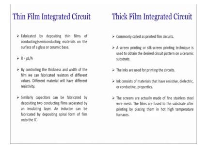
Then what is difference between thin and thick film technology thin film technology using that we can deposit conducting semiconducting materials on the surface of a glass ceramic base or an oxidized silicon.
