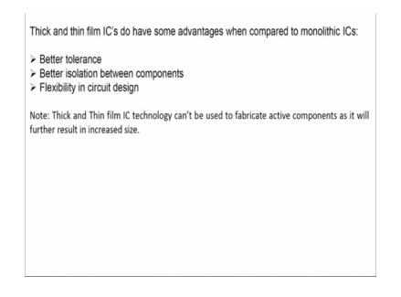
Some advantages over the monolithic ICs are better tolerance better isolation between components flexibility in circuit design. These are the advantages, you see when we were using monolithic integrated circuits the flexibility was an issue here, we can design the thin and thick film ICs on a flexible substrate that is a advantage.
