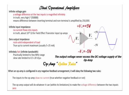
So, then we have seen ideal op-amp an ideal op-amp has few characteristics such as infinite voltage gain infinite input impedance, 0 output impedance infinitely fast of course, op-amp has 2 golden rules. We had discussed those golden rules first is that the input to the op-amp draws no current, and second is the output will do whatever, it can to make the voltage difference between 2 inputs 0 these are the 2 golden rules.
