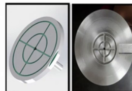
Figure: Wafer holder of 5": designed (left side) and fabricated (right side)
