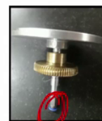
Figure: Wafer holder with vacuum connector
