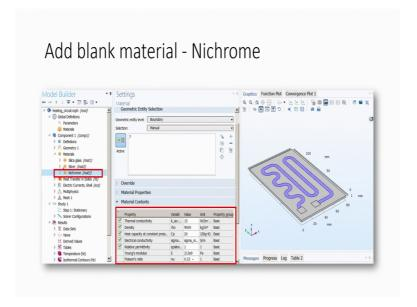
You select the material for the heater which is your nichrome. You can see the properties of the nichrome which is thermal conductivity, density, heat capacity, electrical conductivity, relative permittivity and of course, you have Young's modulus and Poisson's ratio.
