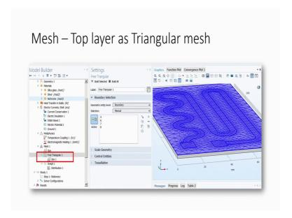
And then, you go for the temperature coupling electromagnetic heating followed by the meshing so, you are creating a mesh, top layer is a triangular mesh, you have swept mesh, the top meshing layer.
