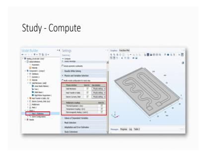
Followed by if I want to go for a stationary then I can select soil mechanics, heat transfer, electrical current and the multiple physics couplings would be thermal expansion, temperature coupling and electromagnetic heating. So, combining all this things together I can understand what is the stress across the film?
