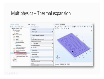
Then, we need to see what is the thermal expansion? So, you can see here the thermal expansion properties we can select for the materials. So, coefficient of thermal expansion material the strain reference temperature is about 293.15. For the selected material, there is a thermoelastic imaging and damping for this particular material and the coupled interfaces for this particular subset is heat transfer in solids and solid mechanics.
