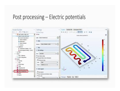
Now, we have taken an example of a heater where we have seen how to understand the electrical potential or the temperature, right when we apply a certain voltage to the pad.
