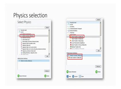
Then, you go for electrical currents and the heat transfer, there will be the physics that you have selected because we are using heater that is why you have selected the heat transfer. We have to apply a voltage that is why we have select a electrical currents.
