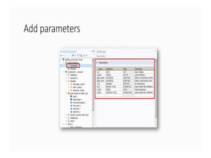
And then, you apply the parameter what will be the parameter that you are applying voltage, thickness, conductivity of silver. Because, you know what is the conductivity of the contact pair, conductivity of the nichrome and then you have to understand, what is the temperature of the room what is a heated air, what is a fluid heat temperature and what is the heat transfer coefficient?
