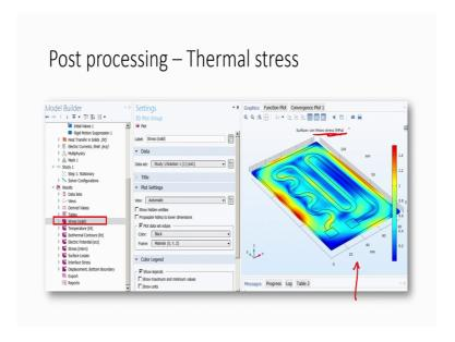
So, this is very important because what we have seen is the heating and what we have seen is the electrical potential. Now, I want to know because of the heating of the chip, what is the stress across the resistor. And you as you see the stress across the resistor as
