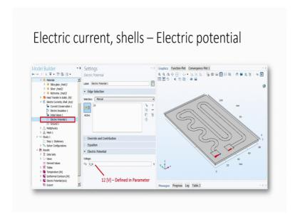
And, heat flux to one front and back side. Then, you go for the electrical potential where you are applying. So, you are applying between this terminal and this terminal so, you are applying 12 volts here ground here.
