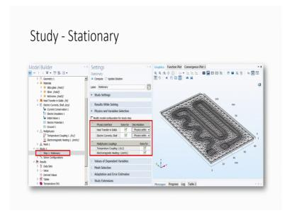
You have selected all the parameters, heat transfers, electrical current, temperature coupling, electromagnetic coupling, right and then you see what is the temperature.
