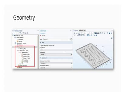
So, when you select this parameter and then you use the; so, this parameter will be applied to this particular section, where you have a glass plate and you have a heating film alright. So, here we have selected a little bit bigger heater just to explain you up and when you select the geometry you have a multiple options here also. So, what is square 1, square 2, filet 1, filet 2 is that plane geometry or not?
