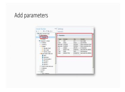
So, what is the parameter that you are using for your for your selected design? In the in our case what is the selected design? The selected design is a heater. So, what we have to understand? What is the voltage that you want to apply? So, here is a voltage. Then what is the layer thickness? Then you are selecting here, what is the layer thickness? About 10 micrometer, 12 volts is the maximum voltage.
