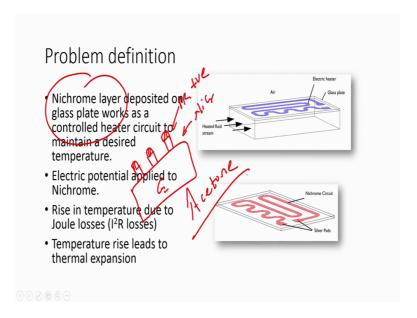
When you this wafer in acetone not deposit sorry you dip the wafer ok, you dip the wafer in acetone what will happen? It will strip off the photo resist. So, it will strip off the photo resist. When you strip off the photo resist, what will happen? You will you will be having a nichrome heater on the glass that is what is shown here that what is shown here.
