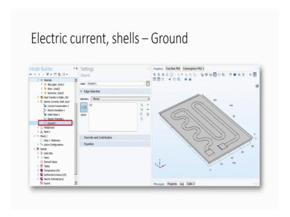
See this ground. So, here earlier if you see on the pad 1 that is the silver pad right here which is a blue color line you are applying 12 volts this one ok. And then you apply where is a ground, so, ground is right over here right. So, we applied electric potential between two pads followed by temperature coupling right and then electromagnetic heating.
