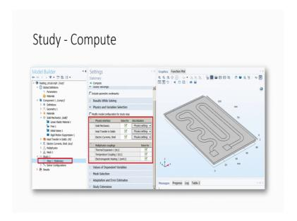
So, let us just understand until here for today's class and we will follow with another module in which I will explain you further details. So, for today's class what we understood is that there is a simulation tool called COMSOL multiphysics using which we can understand the effect of voltage on the on the heater and what is the temperature distribution over the chip when form a particular design.
