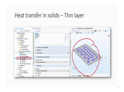
So, thin layer 1 we have selected, we have selected coordinate system as global, layer type we want to know is thermal thin approximation right.
