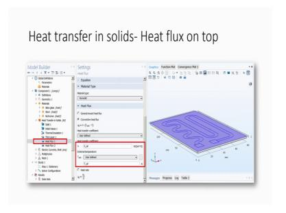
And then when you select heat flux you want to see what is the heat transfer coefficient, which is h air and if you want to see the temperature it will be T air.
