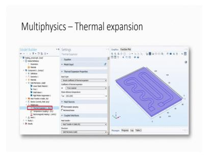
Something goes for thermal expansion right. So, this is what we have seen is you see here lets us go for here heating right and then you can see the electrical electric potentials followed by solid mechanics in which you can see the rigid motion suppression, after that there is a thermal expansion followed by a stationary and so on and so forth.
