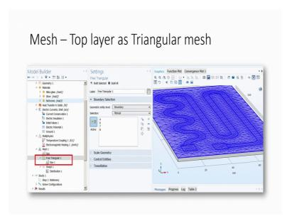
Then we have to create a mesh right. So, if the mesh size is extremely small it will take longer time and you will get a better result compared to a larger mesh you need to use a smaller dimension in the mesh.
