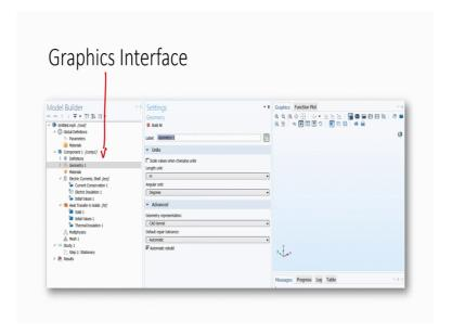
So, let us see once you do that the next step is to select the geometry. So, you are selecting a geometry from the component window and then you can select the length is it in meters, micrometer, the unit in degrees or what if you want to go for advanced geometric representation is using cad and your repair tolerance can be automatic. When you select this item then the next step would be that you have to select the model parameters.
