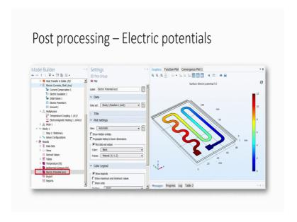
After this the next step would be to see the electrical potential. So, you can see when you apply 12 volts, right over here and this is a ground which you can see here, how the electrical potential varies across the resistor? Across this resistor how the electrical potentials are varying um? So, that is another thing that you can work on you can see ok.
