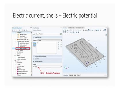
Then electrical potential where you will apply you have to select this boundary this is what we selected and then we have say that here we will apply 12 volts right. So, this is with respect to this. So, this will be grounded and this will be; so, voltage applied between these 2 pads.
