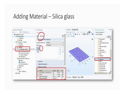
And then what is the material? So, what is the material that is on which you are fabricating the heater, is it silicon or is it a glass or is it some polymer? So, we have a option of selecting the material where you have selected here silica glass. You can see here lot of material options are there.
