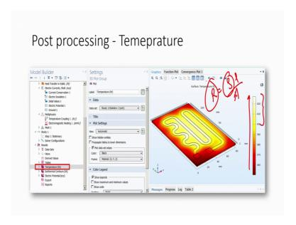
So, now, if we see the effect of the voltage, 12 volt to this particular chip on which there is a heater, you will see that the temperature distribution right over the chip and as you can see the maximum heating that is about 420 degree centigrade is in this particular region. There is another parameter you need to understand why the heating is more in a particular area compare to other area. You can also see that it is kind of uniform in the centre right.
