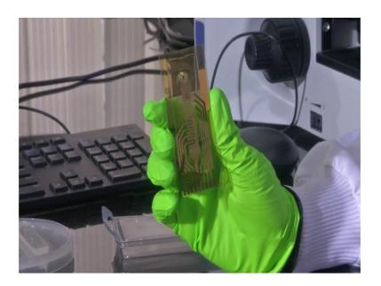
So, when I tilt it, you can see the screen printed electrodes, you can see the screen printed electrodes here see. So, if you see if you observe, these are not very micro dimensions, electrodes are actually even 1 mm thick electrodes. If you see the these are also again interdigitated structures, if you see this is the first electrode and these are sub interdigitated structures, this is from applied bio physics.
