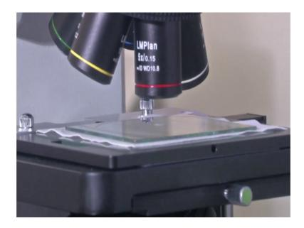
So, before we see anything on the microscope, first we should start with the slowest lowest to know the features properly ok. So, let us look at the screen now so, I have kept before looking at the screen. So, the sample is loaded I have kept the 5 x magnification microscope focused it on a electrode structure now, let us look at the screen.
