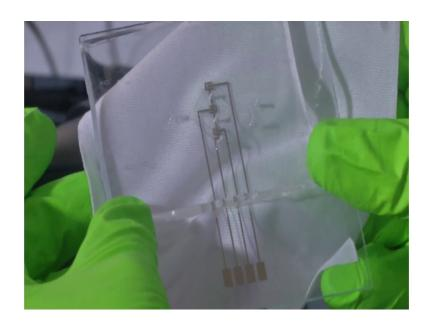
So, we have the glass substrate below, the electrodes are there you can see it right, the golden colour electrodes are there electrodes are below and to that glass substrate with the electrodes, we have bonded the cut nicely cut PDMS channels. So, channels are there visible here hope you can see may not be able to see, but you know that you have seen this before. So, there are channels here so, the channel the PDMS is bonded onto the glass with the electrodes.
