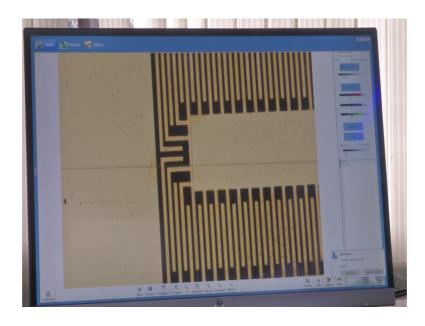
So, I am adjusting the focusing so, now, the focus is adjust, adjusted. So, now, you can see it is at 10 x magnification. You can nicely see the electrode pattern; I will just move the sample around so that you can appreciate the features ok. So, these are the electrode structures if you want to see in much more detail, can go to the next level of magnification which is 20 x.
