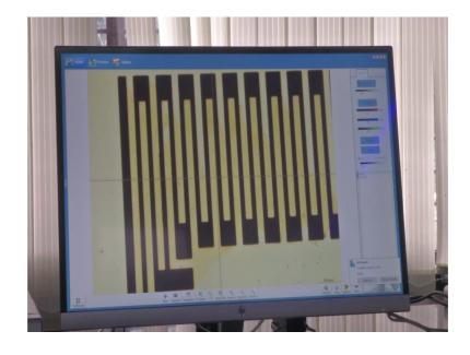
So, this is 20 x magnification ok at 20 x magnification, you can see the exact finger like pattern of the electrodes correct, how the inter digitated structure which we have covered in the course, how they are structured see one pattern of electrodes are coming from top, one set of electrodes are coming from bottom, but they are not in conduct they are like this, they are not in conduct.
