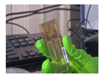
So, this is a microfluidic chip, this is not something that we have fabricated, it is made by company called applied biophysics. But, they wanted to show it to you because this is a very interesting microfluidic chip which is actually fabricated at very low cost, it is made of plastic and it is flexible. See I am flexing it, nothing happens with there we saw the sensor made of glass so, this is made of plastic, everything is made of plastic actually.
