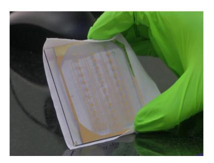
So, let us just see that now, we have a series of electrodes that have that have been formed on a glass substrate. Here, you can see a series of electrodes exactly 30 number of electrodes that we have fabricated here in our facility on glass substrate.
