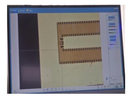
So, you can see in the screen, this is at 5 x magnification. So, this is the electrode the square shape that you had seen where I told there are inter digitated electrode structures.
