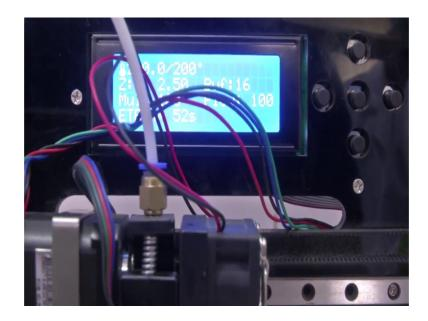
So, you can see it here 4 minutes 47 seconds is remaining. So, the extruder is printing very fast. So, this is this is a 3D printer that we have assembled in the lab. Actually we have procured the individual components of the 3D printer and the enthusiastic members of our lab actually assemble the 3D printer together because of which we were able to make it work in much cheaper cost, even one-tenth or one-fiftieth of the actual cost of 3D printers that are available. So, it is getting printed.
