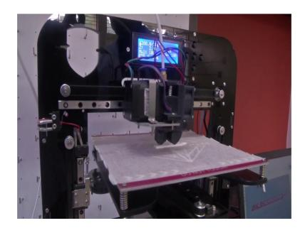
So, the first layer base layer is formed. You can see that pattern getting formed here. So, you can see that it is trying to print it with maximum precision as much as possible. So, it if you see the display, you can see that estimated time remaining is around 7 minutes 39 seconds.
