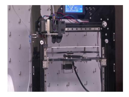
To start off with the printing, so what happens is the printer will go to its home state or zero state where x equal to y equal to z equal to 0. And then, align itself before it starts printing. So, it takes little bit of a time to start. Let us just see it.
