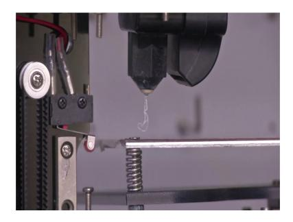
So, it is testing out how if the material is coming out properly. So, once it is melting that it is coming out properly, it is starting the print.
