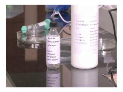
So, it is basically PDMS, it is effect it is a 1 kg bottle. We will use very less quantity of that around 50 ml. Then this is the curing agent. So, this is another chemical. So, this curing agent is what will make the PDMS become solid after sufficient time.
