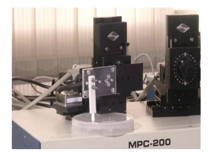
Let us look at manipulator a now so, we had seen manipulator a, we have seen that there is a indenter holder for the manipulator correct and we have attached this indenter holder here which has lot of holes here, which will allow you to attach several indenters to this port ok.
