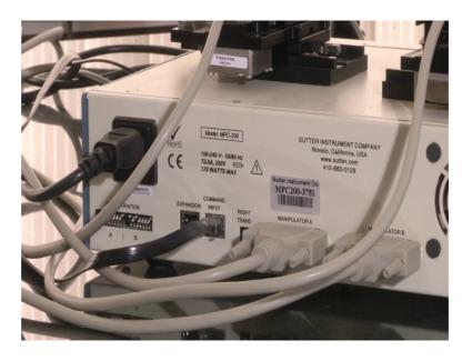
So, I have connected it back this is a command input port. So, let me just show the control unit to you now ok, this is the back side of the control unit ok.
