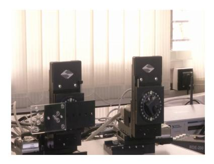
So, this is the manipulator so, I am just tilting it a little bit. So, if you see here in the manipulator micromanipulator will be able to move in x y and z directions.
