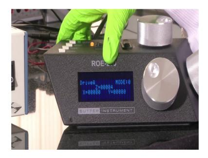
So, you can go up there it is showing that it is mode 0; mode 0 is visible, drive a is visible, then you can see is z, x and y values. So, z, x and y can go from 0 to 25000. So, z, x and y can go from 0 to 25000. So, I am just making it back to 0 now z, x and y are at 0 ok so, one is drive what is the manipulator that you are driving and then one is mode and one is the z, x and y values.
