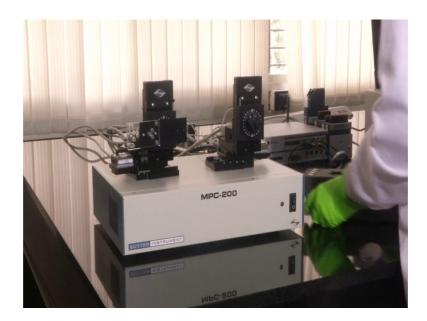
So, here we have the micromanipulator system ok. So, this white platform that is there is a main unit and this black platform that is there is a right is a control unit, control unit forms like their brain or the main heart of the manipulation system as far as controlling goes and the manipulators themselves are these 2 black platforms.
