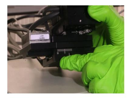
Now, to see the x scale I am just tilting it so, I think you can see the x scale here below there is also 0 to 25. So, we have 25 mm of movement in the x direction, in the y direction and in the z direction clear. Now, that is for the coordinate movements. Now, if you see closely so, in this manipulator we have attached somethings let us just check the manipulator b, this both are same dimensions are there 0 to 25, 0 to 25 and here if you see it closely in the back side it will be there 0 to 25.
