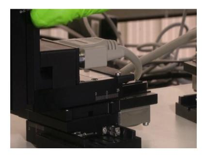
So, if you see here this is the y direction; y direction scale can you see the scale here from marked from 0 to 25. So, that shows that the manipulator can do movement of 0 to 25 mm ok, 0 this total is around 2.5 centimetres or 25 mm. So, it can travel in the y direction through 25 mm that is the scale or range of movement of the y movement of the manipulator understood.
