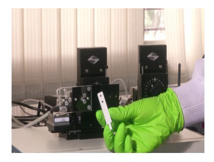
So, we have 3 D printed using 3 D printing technology, we have 3 D printed quite a big a macro scale indenter so, that is very visible to you. So, this is the attaching part of the
