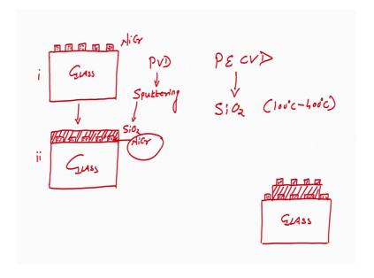
So, what is alternative, alternative is either you go for PVD, which is your sputtering or you go for plasma enhanced chemical vapour deposition. Since, the plasma enhanced chemical vapour deposition; the silicon dioxide can be grown from 100 degree centigrade to 400 degree centigrade. As low as 100 degree centigrade, you can grow silicon dioxide.
