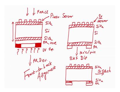
Then for that we have to use photolithography. And if you are seeing the last video in the photo lithography section, you will be able to see how to perform front to back alignment, and get this kind of design. In that case, we have to spin coat photoresist on the backside backside of the vapour right. And then, we perform a photolithography by loading the mask right.
