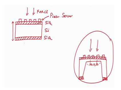
So, let us see how we can use this one for our this particular example. So, if you see the screen, if I have an oxidized silicon substrate, you understand this ok. Now, you guys know how to pattern a micro heater interdigitated electrodes or any pattern any given pattern right. So, we have silicon dioxide, we have silicon, we have silicon dioxide.
