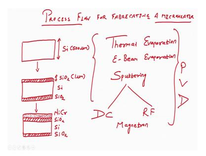
So, let us take an example of a fabricating micro heater on and oxidize silicon wafer. And then, you will also see how we can design a micro heater on a glass all right. So, what we are learning today, we are learning the process flow process flow for fabricating a micro heater process flow for fabricating a micro heater. So, what is this process flow and then a micro heater ok?
