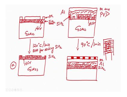
So, when you develop photoresist, you will get glass, heater, photoresist, nichrome, photoresist, silicon dioxide, glass right. After you perform, this development stage or developing photoresist and unload the mask, you will have this particular pattern.
