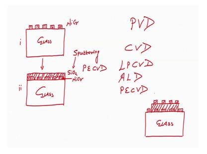
So, let us see on the screen. If that is the case, what we require, I will draw it here, what we require; this is what we require as a final device. We take example, like we have a glass as a substrate right, on the glass, we have micro heater ok. And on the micro heater, let us draw like this. On the micro heater, we want to have an insulating material. On insulating material, we want to have interdigitated electrodes.
