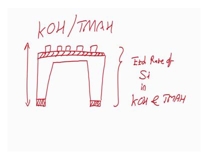
So, what will be the next step, next step would be to etch silicon. So, after this if I keep the wafer in silicon etchant in silicon etchant, what will I have, what are my silicon etchant, my silicon etchant are potassium hydroxide or TMAH right. So, if I did the wafer in silicon etchant, what will I have, I will have.
