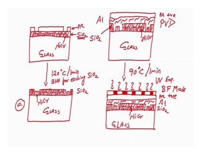
So, now you have bright field mask, that we have loaded positive photoresist, aluminium, silicon dioxide, we have micro heater, and we have your favourite glass substrate, can be your is can be my favourite also does not matter ok. After this, what is the next step next would be next step would be UV exposure next step would be UV exposure.
