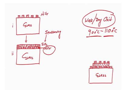
In PECVD so in LPCVD, what was the case LPCVD if you remember, the oxide that is grown like wet oxidation wet or dry oxidation the temperature was 900 degree centigrade to 110 degree centigrade correct 900 degree centigrade to 110 degree centigrade. So, if I use if I use this technique, then my nichrome will get melt nichrome will melt right, because this is extremely high temperature, or so that is why, we cannot use wet or dry oxidation technique to grow silicon dioxide on nichrome.
