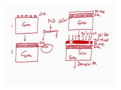
So, next step would be next step would be to spin coat photoresist right spin coat photoresist. Why we are using this, to remove the silicon dioxide from the contact area right, you see here ok. So, this is our photoresist, silicon dioxide, nichrome nichrome, glass correct positive photoresist positive photoresist. Now, after this, we know we have to softbake 90 degree 1 minute hot plate.
