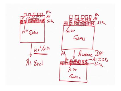
So, when we perform UV exposure, there is a bright field mask, what you will obtain, you will obtain a glass wafer, silicon dioxide, glass, nichrome, aluminium, photoresist, ok.
