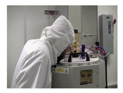
We have a flash light, change the machine to check that the wafer has been load properly sure; we have to turn on the light and check through the window the wafers prescribe properly and the clamps inside the machine are holding it in place.
