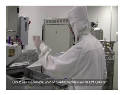
And once we press, then we have to wait for the role of chamber to which a atmospheric pressure. I have once the transfer chamber is on the atmospheric pressure we can choose we open it. Now, we will charge the desire wafer into the chamber, assume, we say like usually the wafers have the flat and closing characters we have a small line.
