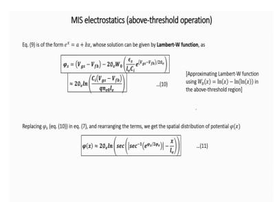
Which can be approximated as this particular expression here. And the surface potential therefore, is and the potential through the semiconductor not the surface potential, the potential through the semiconductor is given by this particular expression. The surface potential in particular is the potential at x equal to 0.
