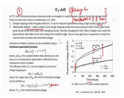
And once C is a very unique phenomena in disordered semiconductors which is something called as the threshold voltage shift. So, what is this mean? So, in the case of crystalline silicon MOSFETs the threshold voltage was more or less a fixed quantity. I mean we once you know the threshold voltage at the MOSFET you used it for modelling your circuit behavior. But in the case of disordered semiconductors when a MOS when the thin film transistor is an operation.
