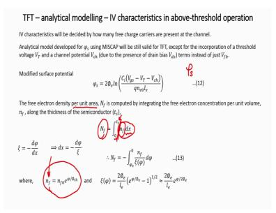
Now, the next step towards modelling is now, we have the potential function and we have this surface potential. Now the surface potential determines the free carrier concentration per unit volume. Because of free carrier concentration per unit volume is
