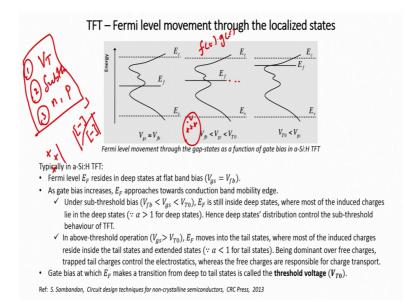
Now how does a thin film transistor work? Now as we so, what we have to look at here is the density of states picture. So, let us say we have a we have applied a gate voltage we built a thin film transistor and we start throwing in positive charge on the gate.
