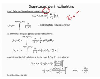
And on the other hand if the alpha is less than 1 which so, which happens to be the case in the case of tail states.
