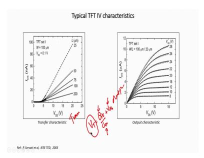
And this plot here shows that typical transfer and output characteristics for a TFT. Now since the threshold voltage is nothing but the trap charge by Cox plus Vfb this is a trapped charge per unit area divided by Cox plus Vfb the threshold voltage ends up being a very dynamic quantity.
