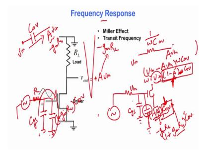
And since and you can represent you can if you want to represent the capacitor as an effective resistor you can do, so by simply replacing it with it is an impedance of 1 by omega C overlap so that is basically your resistance. So, you have a current of V in the voltage drop across this is V in minus A V in into omega C overlap is basically the current through the circuit or in other words you have a current of V in into 1 minus A omega C overlap through the overlap capacitor.
