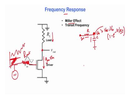
But let us just keep it simple we will say that there is a sensor and the sensor is throwing out you know these high frequency signals, but sitting at a large DC voltage to keep all this in saturation. And the sensors got some output impedance and it is sending these signals here. Now, when these signals were very low frequency, we really did not care about it, because we knew that the MOSFET could easily respond to these low frequencies, but now we need to be very careful.
