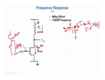
So, let us say there was another amplifier here and we know that we know how to calculate Z out. So, it has got some output impedance and that amplifiers sending out some signals and it is being sent to this amplifier. So, it could be any situation.
