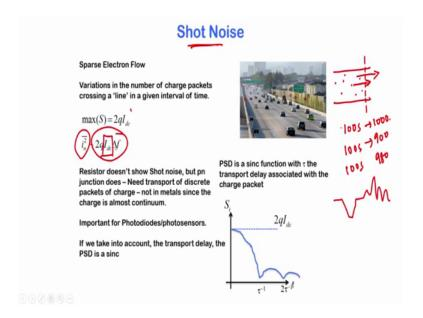
And then you have something called as short noise. So, I am just going through this just to give you a glance through the devices ok. So, here you can again compare it to traffic, but traffic which is very sparse ok. So, let us say you have a electrons moving in a conductor a moving in a in a device and the electrons are very sparse.
