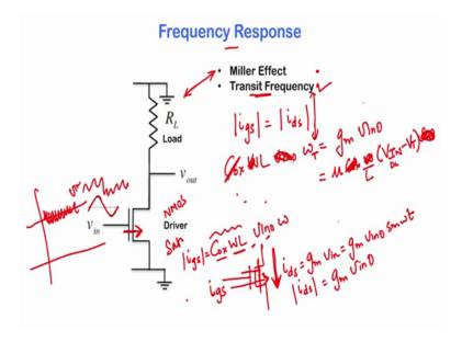
So, the magnitude of i g s is going to be the capacitance of the gate capacitance which is nothing but C ox into WL, so that is going to replace the term C here. Cox into WL let me just remove this, because we do not need that into V in o into omega so that is your total gate capacitance. This is the capacitance per unit area into the area, which is W into L into V in into omega, so that is the total gate current.
