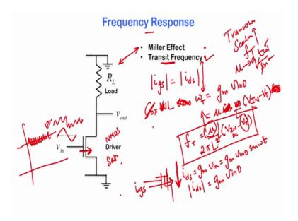
And if you write it in terms of the frequency in hertz, if you say f T, then you divide this by 2 pi. So, this is a very key parameter and any technology ok. So, it is telling you that at a certain frequency that the gate input gate current will match the drain to source current and that frequency is given by f T, which is mu by L square into V IN Dc minus VT.
