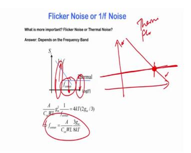
And finally, the very last topic is something it is got to do something called as a corner frequency with regards to noise and the MOSFET. And what is corner frequency? We know that thermal noise. So, in a MOSFET there are two key components of noise, we have the thermal noise and we have the flicker noise. And thermal noise is rather frequency independent it is almost constant all frequencies. And therefore, it is called
