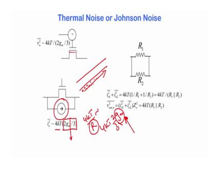
Now, in a MOSFET in conduction, you do have thermal noise when you have an inversion channel formation, but once the inversion layer is formed you have a large number of electrons between the source and drain. And therefore the MOSFET has thermal noise through it. So, when we talk about MOSFETs and circuits we must take care of introducing the thermal noise, if you are worried about the noise behavior.
