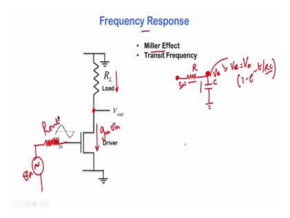
Now, R interest here in this study on Miller effect has got to do with the input sensor. So, let us say there is a input sensor, which is sending in all your V in signals and those signals are all coming here, but the sensors has got some resistance it is got some output resistance, which is normally the case it could also be a previous amplifier.
