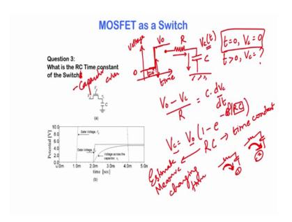
But, essentially the time constant is a useful parameter that gives you an estimate; it is an estimate or a measure of the charging time of the circuit you know. If you want to compare two RC circuits you compare two RC circuits, and you say that this one has got a smaller time constant than that one, which means to say that this circuit will charge faster as compared to circuit 2 ok, which means to say that circuit 1 is faster compared to circuit 2.
