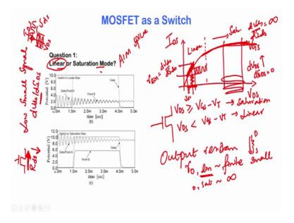
So, so here is the simulation ok, so the answer to this question is we want the MOSFET in linear. And to prove the point here is the simulation, which is done using AIM spice, so which is the software ok. And the simulator takes into account this circuit, so we are simulating this circuit here shown here.
