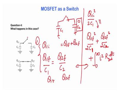
So, so according to charge conservation, you had up get one equation, which is basically this. And after at t equal to infinite, after you have short circuited this at t equal to infinite, these two points must have the same voltage ok, they cannot have different voltages, they are short circuited. And at t equal to infinite, they must have the same voltage.
