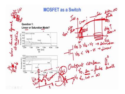
So, the first question ok. If I were to use the MOSFET as a switch and I want low I want low small signal resistance across the switch, do I bias the MOSFET a linear mode of operation or saturation mode of operation that is the first question. So, just to recollect what is the linear, what is the saturation mode of operation?
