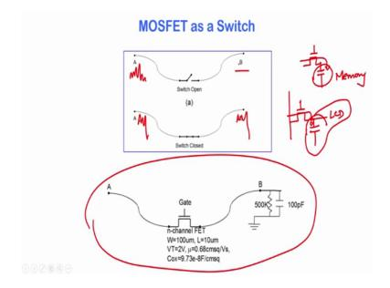
So, let us start off by looking at the MOSFET as a switch. Again, we are going to go back to a traditional example that we used to introduce transistors, which is I have point A and point B. And I want to send a message from point A to point B, and I need a switch in place. So, when the switch is closed, the message here gets to point B; and when the switch is open, nothing happens at point B. So, here is a more complete circuit.
