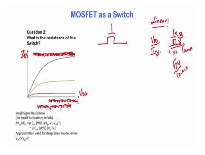
We are not talking about resistance measured as V DS by I DS, no because if it is V DS by I DS, even the saturation mode in the saturation mode, the MOSFET does have a finite resistance ok. You have let us say a V DS of 5 volts. And let us say the V GS is whatever 3 volts, and therefore the MOSFET is in saturation.
