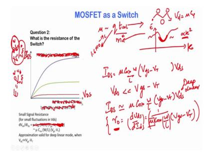
So, the value of that, since we have biased the MOSFET in linear mode operation, what is I DS, I DS is mu Cox W over L into V gs minus V T minus V ds by 2 into V ds. And if my V ds is much much smaller than V gs minus V T, we could say that we are going to ignore this term. And therefore, I DS is approximately mu Cox W over L into V gs minus V T into V ds ok. So, this is something called as a deep linear, I mean it is a very very linear operation. V ds is much much smaller than V gs minus V T.
