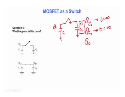
Now, here is another useful circuit, but although this really does not connect us to our device physics, nevertheless it is a useful circuit for all of you to know ok, which is basically you have a capacitor that is charged with some charge Q 1. And you have another capacitor say C 2, which does not have any charge in it. And you use a MOSFET or any switch for the matter. So, although we are talking about MOSFETs as a switch,
