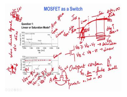
But, let us look at the voltage at point A ok. The voltage at point A is the this is 500 kilo ohm that is point B, and this is point A, this is where the signal is coming in, so that is 10 volts that is V GS. What is V DS? So point A has got a signal that looks like this right. And what is the DC value of that signal that somewhere here and that is about 9 volts.
