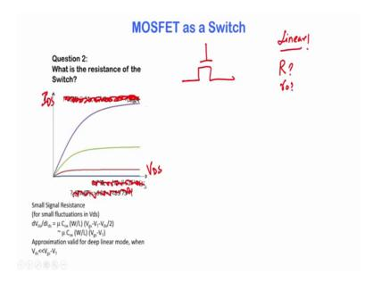
Now, what is the resistance of the switch ok? So, what do you mean by the resistor, what is the resistance of the MOSFET switch? So, do forgive this plot having all these scripts, because this is the image that is transferred from a Mac to a PC, and it generally happens to have these kinds of errors.
