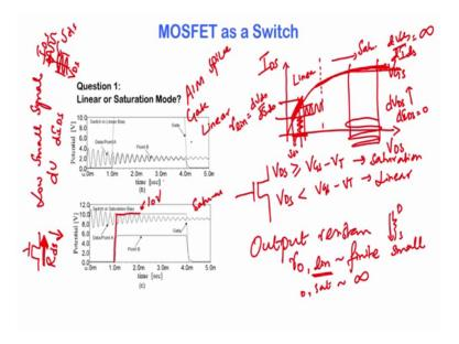
Now, what about keeping the MOSFET in saturation mode of operation ok? Now, this is the case, where the MOSFET is in saturation mode. How do we know it is in saturation mode? So, the gate voltage is still the same; when it is on, it is still 10 volts.
