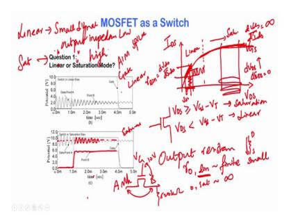
So, in linear mode operation, the MOSFET has the small signal output impedance of the MOSFET is very low. And in saturation mode operation, the small signal output impedance of the MOSFET is very high. And therefore, we want the MOSFET biased in linear mode operation for use as a switch ok. So, we have decided it is linear mode operation.
