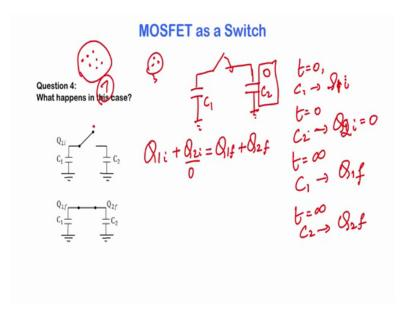
So, if you use charge conservation what is the total charge, so the total charge is Q 1 initial that was the entire charge in the system, because Q 2 initial was 0. So, this is simply, so this is nothing but 0, and that must equal the final charge in the system.
