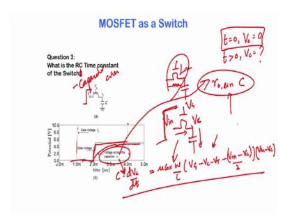
So, if you have a MOSFET operating in linear mode operation, and somebody I asks you is to what is the small signal capacitance a small signal time constant of the MOSFET, it is simply r o linear into the capacitance of the capacitor, it is an approximate model. And what is the approximation, we have linearized the MOSFET.
