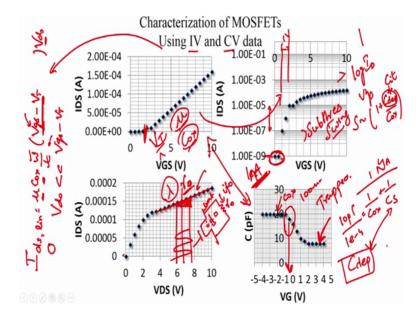
An ideal MOSFET the current supposed to be constant with Vds, but it is because of channel length modulation that you actually have a variation in current in the MOSFET. And therefore, this is a useful plot to identify your channel length modulation parameter and the effective output resistance of the MOSFET, ok.
