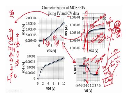
So, now we, we have obtained VT, Mu and C ox and we can now plot the same transfer characteristics on a log I D versus VG scale in order to obtain look at the sub threshold behavior of the MOSFET. So, we know VT, so, we know that in and around let us say about 2 Volves, ok. So, after 2 Volves, the MOSFET enters above threshold operation. So, here it is all given by a square law characteristics and below this below this we know that we are in sub threshold region.
