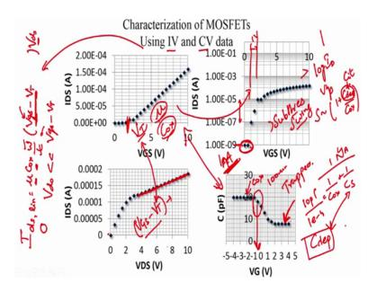
So, in saturation mode we firstly, identify the point at which saturation occurred. So, technically this should be VGS minus VT, but it could be offset by some amount because if you remember the bulk charge theory predicts a different saturation voltage as compared to your square law the simple model.
