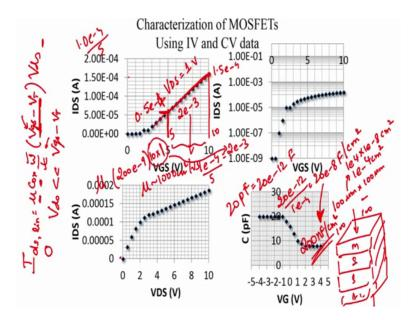
So, firstly, let us say we performed the most capacitances on MOS capacitor having 100 microns by 100 Micron. Those are the dimensions, which means that, that was 100 microns that is 100 microns and you know that was the MOS capacitor that we used, ok. So, as a metal insulator semi conductor back contact. So, what is 100 microns by 100 microns, we would like to represent everything in terms of centimeter square.
