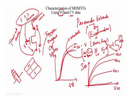
So, essentially let us say you have made a MOSFET, ok. The very first characteristic characterization technique is the most essential, which is using your IV and CV information to extract key parameters of the MOSFET.
