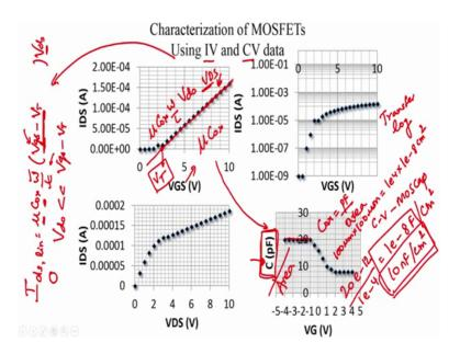
So, at the end of it, we should obtain a family of curves that look like this. So, here I do not, I have not shown a family of curves, but we are we are seeing just one set of one data set, ok. So, here we have the transfer characteristics, we have the transfer characteristics plotted on a log scale. Here we have the output characteristics and here we have the C V characteristics of the MOSFET. So, how do we extract all the parameters required by using this IV and CV measurement?
