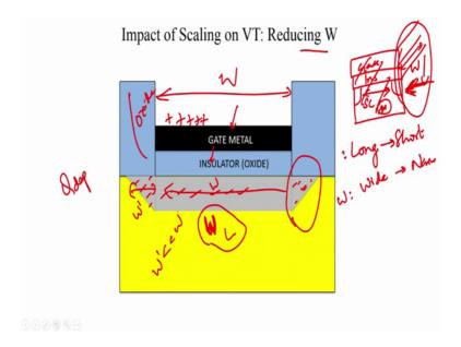
Now, for a very wide device this extra work done, really does not make any difference ok. It is a very small percentage of this total channel width. So, this W dash is a very small percentage of W, but for a short channel device it becomes a very significant portion ok.
