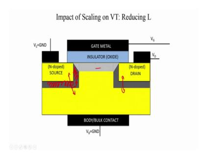
Now, what happens; if start reducing the device, if you start reducing the device ok. So, here I had a nice picture and I did not use it. This dark region shows, the portion of the, portion depleted by the PN-junction, whereas, the gray region shows that, portion depleted by the gate.
