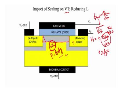
So, the gate can be said to be depleting, the entire area, which is about W into L ok. So, that is the area, the gate has to depleted.
