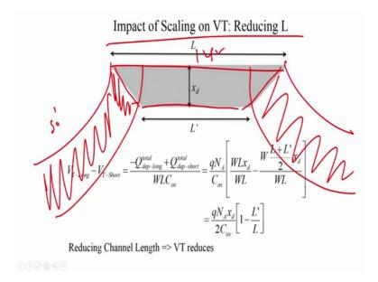
So, let us just take the depletion region of the gate the region of the semiconductor depleted by the gate. So, that is where your source drain would be and that is how the depletion region would be around. Your source drain and this part of it is all taking care. It is all depleted by the source and drain and it is only this region. Here, that is depleted by there gate and that is the insulator ok. So, that is the picture.
