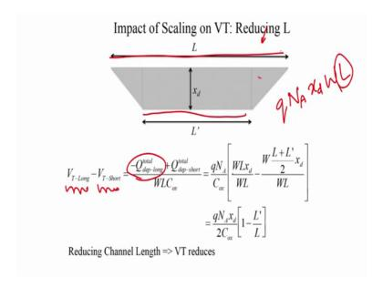
So, not per area or volume not this; so, what is the total charge? So, let us take a difference let us say. Now, what is this area? You know, how much of this volume, this gate depleting what is the total depletion charge, what is the threshold voltage of the long channel device minus the threshold voltage of the short channel device, in the case of a long channel device ok. This, it is almost the total charge is almost it is going to be q N A x d, that is a charge per unit
