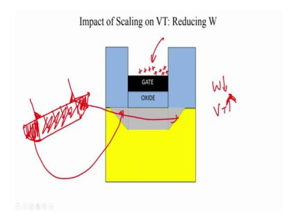
You have a gate you have an insulator here and this insulators are sharp if you look at this edge of this insulator. It is a sharp a corner and this corner is going to have a very strong fringing field. So, that is the way the field lines are going to be present it is going to have a very strong field. And therefore, this is the depletion region, it is you can say it is more like a sector of a circle and then here you have this region that is depleted.
