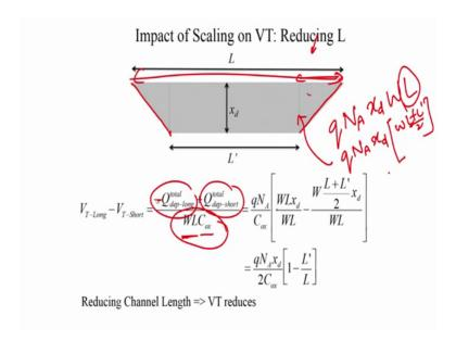
So, what is the difference between the Vt of a long channel device and a short channel device. It is a difference, in this depletion charge minus this depletion charge divided by the total capacitance. So, its capacitors per unit area into WL ok, and this minus sign is there, because of this minus sign is present, because of the all the charge is being negative.
