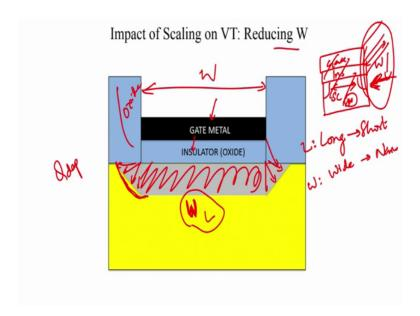
So, once again the answer has got to do with the depletion charge. So, total depletion charge. So, if you look at this depletion profile, yes, most of this depletion, if you look at the total depletion charge all depletion charge spans over a, length of W and of course, the channel length to say, L and therefore, W into L is what is depleted, but then, because of the fringing in the field ok.
