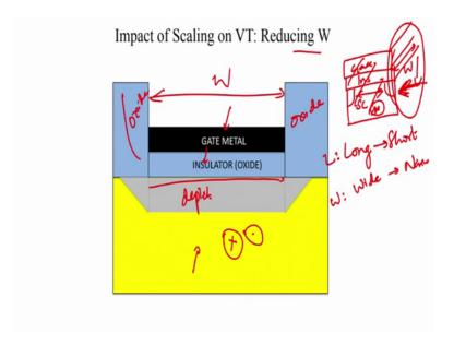
So now, what about the impact of scaling on the of the channel width ok; so, we have your we have the MOSFET which is got the it is the gate insulator semiconductor and you now have, we have discussed the impact of channel length, but what about reducing channel width. So, for reducing channel length, we say it is a long channel device to a short channel device, but for channel width, we say it is a wide device to a narrow device.
