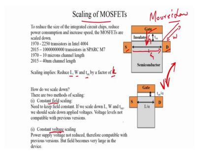
The other idea is something called as constant voltage scale which, in this case even despite your scaling down of lengths the voltages remain constant. In order for you, to continue having compatibility with regards to the power supply required for operation etcetera and; obviously, in this case, the electric fields are going to increase as you scale down the MOSFETs.
