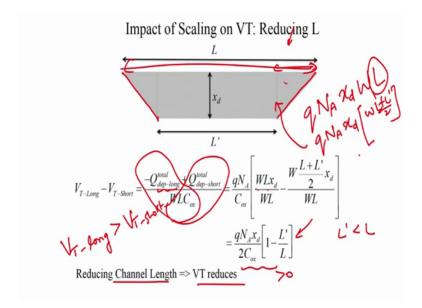
So, this total depletion charge is q N A by Cox into WL x d divided by WL. So, that is this term and q total depletion in the short channel device divided by the total gate capacitance is given by this term. So, essentially this reduces to an expression of this kind and if L dash is less than L, this term is greater than 0, which means the V t of the long channel device is greater than the V t of the short channel device or in other words, if you reduce the channel length the V t reduces ok.
