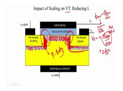
Now, let us look at this depletion term. So, what exactly are we depleting in a MOSFET. So, here you already have a NP-junction. So, this is a p-type body; So, you have a n-type source a n-type drain and you have a P-type body and you already have a depletion layer here, because of this diode.
