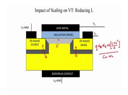
So, what is let us call this as L double dash and capital L, and what is the depletion charge. In this device it will basically, be your q N A I am just taking the magnitude q N A x d into W into the area of this trapezium it should be L plus L double dash by 2, and that divided by the total gate capacitance is essentially going to be. Let us get rid of the WS its essentially going to give you q N A x d by C ox into 1 plus, let us say 2 C ox 1 plus I double dash by L.
