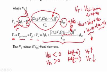
Metal Oxide Semiconductor Field Effect Transistor Improving the Model: Body Bias
