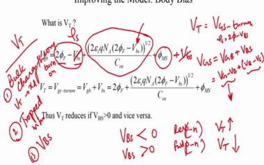
Metal Oxide Semiconductor Field Effect Transistor Improving the Model: Body Bias
