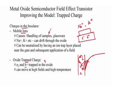
So, these are electrons and holes that are trapped inside the insulator. So, let us let us view the situation little better. So, if you if you remember, you have your insulator and you have the band bending in the semiconductor and you have these electrons here. And these electrons are all basically you know they are all they all have their own wave function.
