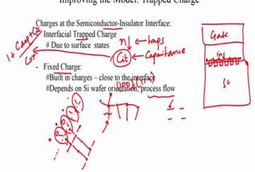
Metal Oxide Semiconductor Field Effect Transistor Improving the Model: Trapped Charge
