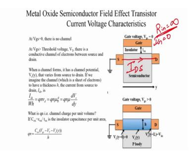
So, if you talking about P channel device, if you talking about the N channel device or an NMOS you have a P type semiconductor and you have electrons there and the electrons and the drain is going to be at a higher potential.
