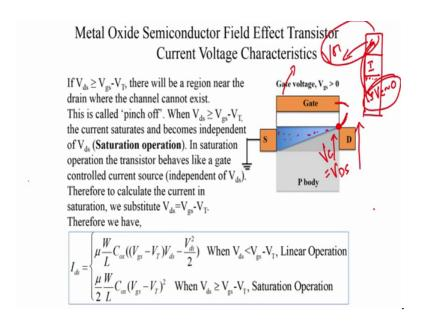
There are electrons every other region is inverted, but just this end near the drain is you do not find electrons because the V g V gs minus V T is now no longer greater than the channel potential. Your V gs minus V T minus channel potential has become equal to 0 and therefore, qn has become equal to 0. So, this end is now pinched off.
