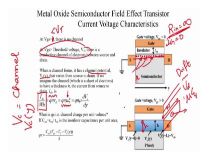
So, we can write this little equation down, which is ids by W h is the current density and that is equal to qn into the drift velocity, but what is drift velocity? The drift velocity is nothing, but the mobility times the electric field. So, we can rewrite that equation as qn
