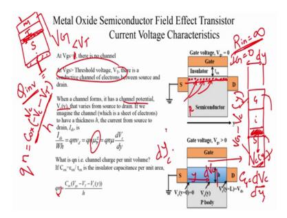
So, we have made this implicit assumption of low Vds and we have assumed we have derived the current voltage characteristics for that condition ok. Now so this region of operation is something called as linear mode of operation ok. So, it is a technical term.
