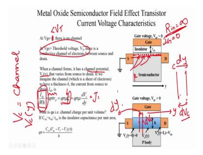
So, you have q n mu dVc by dy as your current density and that is equal to your I ds by Wh ok. Now in order to identify I ds we need to now calculate what is n ok.
