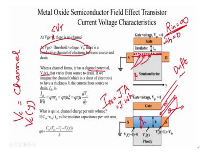
So, all migrating from the source to the drain; so, what is the total current? The total current which is your I ds is basically this current density into the area of cross section and what is the area of cross section? It is basically W into h where W is the channel width and h is your thickness of this electron sheet ok.
