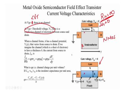
Let us just take with the P type semiconductor and then N MOS device or an electron channel being formed at the interface during inversion.
