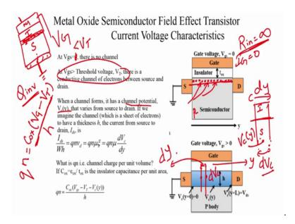
So, we had the MOS capacitor which was a metal insulator semi conductor structure and we had in inversion we had an electron sheet and we had defined that inversion charge is Qinv that was a inversion charge per unit area.
