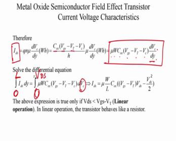
So, if when we did our experiment by moving the voltmeter along the channel we saw that as we moved from the source to the drain L varied x y varied from 0 to L and the channel potential varied from 0 to V ds. So, you apply these limits and solve this equation and you will end up with your current voltage characteristics of the MOSFET ok
