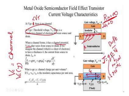
So, what is the drift current density? So, that is J which is the drift current density the current per unit area it is q n V d where V d is the drift velocity of the electrons, n is the number of electrons per unit volume and q is basically your 1.6 into 10 power minus 19 coulombs.
