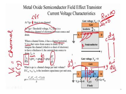
So, you have a section of length dy and the voltage drop across the section is basically dVc. So, what is the electric field across the section it is dVc by dy. So, we replace this electric field term by dVc by dy.
