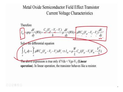
You have I ds is equal to this particular term. So, you have mu WCox V gs minus V t minus V c in a dVc by dVy dy. So, you take dy to the other side and you solve this differential equation. So, you integrate y from 0 to L. This does not is not clear, but this is L. So, as you integrate from 0 to L what are we doing we are moving from the source to the drain and therefore, Vc will vary from 0 to Vds
