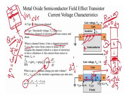
So, you have the channel here, you have the channel here the potential drop across this channel is dVc and therefore, the electric field in that section from here to there is dVc by dy ok. dVc let me just write it clearly dVc by dy that is the electric field and this
