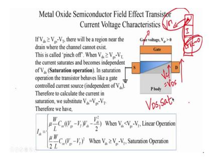
And we now start tweaking up the V ds, we start increasing the drain to source voltage the drain to source voltage at which. So, as you are increase the drain to source the channel potential is increasing. So, let us watch the channel potential near the drain, let us only focus on this section here.
