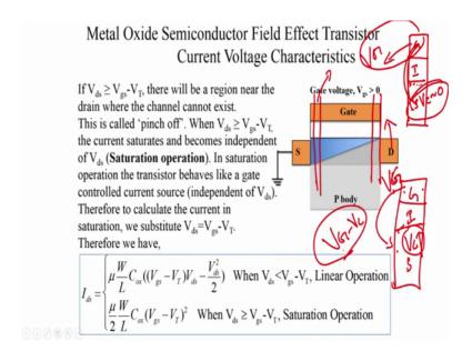
So, let us take a situation where you have gate insulator semiconductor, but the channel potential is very large. Again when can this happen? If this can happen when the V ds is very large the channel potential is very large and now you look at the capacitor you have Vg what is the voltage difference between the gate.
