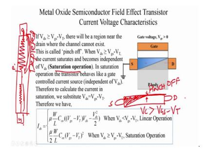
And now if we keep increasing V ds further the transistor we will continue to remain in saturation mode operation. Now in saturation mode operation so what saturates we find that the current through the transistor saturates and I will explain what happens.
