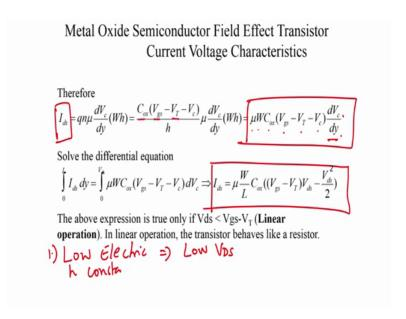
So, that is the derivation of the simplest model for the current voltage characteristics of the MOSFET, but there are problems there are a lot of problems in this ok. So, many assumptions made, many implicit assumptions made. Now what is the first assumption that we have made here? The first assumption is the fact that we have actually used this expression for drift velocity. When is this expression valid? This expression is valid only under low electric fields.
