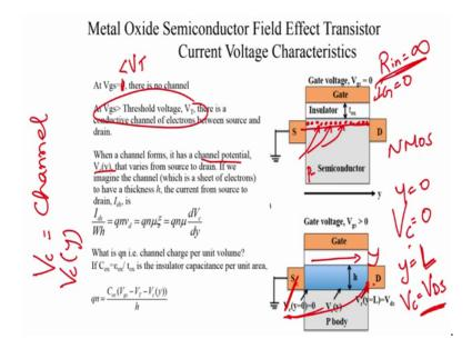
Now let us move ahead, now at some other point the potential difference between these two will be V c of y because its varying with y and as you go to the drain as you approach the drain side the potential here is going to be the same as the drain potential and therefore, at y equal to L which is the channel length V c is going to take a value of V DS which is the drain to source voltage because all these potentials are measured with respect to the source.
