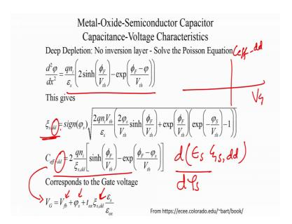
For high frequency characteristics what you do before, we go to high frequency for deep depletion what do we do. For deep depletion this Poisson equation is not correct because in deep depletion there is no formation of an inversion layer.
