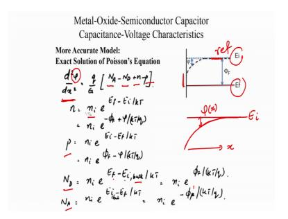
So, the very general Poisson's equation is simply this it is d square psi by d square phi by d x square is q by epsilon into any acceptor ions donor ions, electrons, and holes you cannot get more general than this for a for our case. And the way we are going to define the potential what is this phi.
