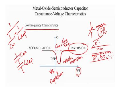
So now let us divide the capacitance voltage characteristics into 3 parts, and we will just go one by one. So, first is something called the low frequency characteristics; what does this mean? This means that I am sweeping my VG very slowly. So, the DC voltage ok. So, let us say we change the DC voltage and then you do a measurement with an AC signal.
