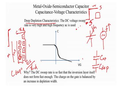
And this case has got to do with the DC voltage and the AC voltage. So, we know not only use a very high frequency AC signal, but the rate at which we are sweeping the DC voltage is also very large ok. So, instead of you turning the knob very slowly imagine the MOS capacitor experiences a rapid pulse, let us say the VG went from 0 to whatever 10 volts and or you know minus 5 to 5 volts within a few picoseconds or a few nanoseconds a very sharp pulse appeared at the gate.
