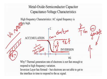
Now, what about the high frequency characteristics ok. So, what is the experiment we are doing here? So, in this experiment you have 2 things to vary, you have VG and you have your e C signal we can pick your AC signal frequency. The VG is varying very slowly you set this you make a measurement then you set this and you make measurement you give the device enough times. So, the VG is varying very slowly ok.
