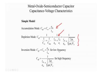
So, a very simple model what is the model for accumulation mode the capacitance is simply C ox in depletion mode this is our capacitance it is a series combination of C ox and C depletion. And C depletion is epsilon s by x d and we know what x d is in terms of the surface potential. So, these are, I am not going to go we are not going to spend too much of time in these relations this is. So, that is the depletion mode capacitance.
