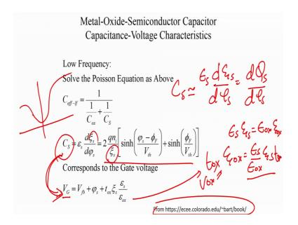
So now we can solve for the exact capacitance voltage characteristics ok. So, these equations are borrowed from this source; so what is our low frequency characteristics in depletion? It is 1 by 1 plus C ox plus 1 by C s and not in d depletion. In fact, this is in general case because we will you can solve it for all voltages.
