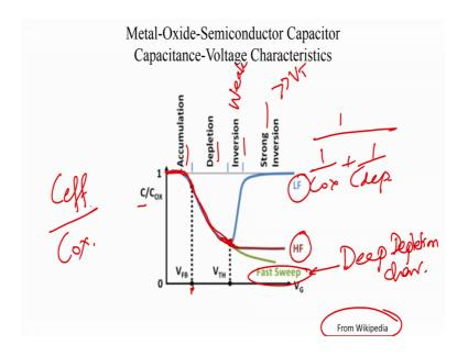
So to summarize all these 3, I have taken this nice picture from an online source and what we are plotting here is C by the C is the effective capacitance of your MOS capacitor C by C ox. So, first is the low frequency. So, we have the low frequency characteristics the high frequency characteristics and the fast sweep or the deep depletion characteristics.
