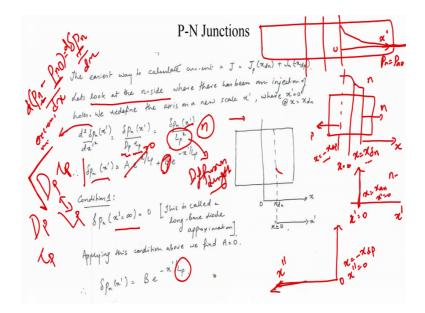
So, let us go ahead and start looking at the proper derivation of the current voltage characteristics of a P-N junction. But before we get to this point we need to understand a bit of what is going on either sides of the junction.
