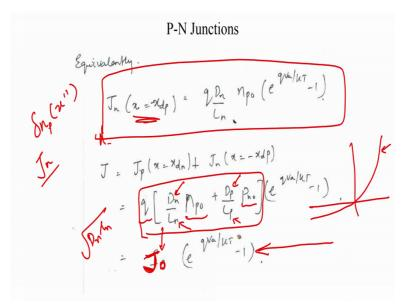
So, once again you solve the continuity equation to calculate the injected electrons into the p side. You find this profile, and then you find your diffusion current due to the electrons. And you will find the diffusion current due to the electrons at the depletion boundary or the p side is given by this expression, very symmetric solutions.
