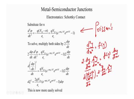
So that is my Poisson's equation so, that is the equation I want to solve to get a more accurate answer ok. And how do we solve this? Now this looks like a tricky equation right you have a d square phi by d x square term on the left hand side and you have got a function of phi on the right hand side. Essentially you have got an equation which says d square y by d x square is some function of y ok.
