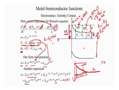
And I want to get an expression for n at say some x. What we are saying is? It is the nth the interface that is n at x equal to 0 times e to the power q phi by k T; which means as phi increases n increases, which is expected because the interface has got very little n and as phi keeps increasing n increases till it approaches the bulk concentration.
