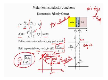
We find that the potential that is phi at x d ok. So, this is my potential variation in space ok. So, that is my phi of x and x keeps increasing and at this point we have your phi of x d. And beyond this the potential remains the same.
