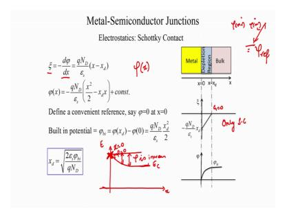
So, where phi is the potential and it is important so all though I am not shown it here, it is important to know how we have defined the potential. So, this is the band bending
