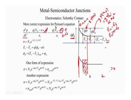
But this is not a constant; it depends upon the potential because it depends upon E c minus E f ok. So, let us identify n bit more clearly. And I will just get rid of these marks here so, that slide is more clear. So, what is n? N is the effective density of states in the conduction band into e to the power minus E c minus E f by k T.
