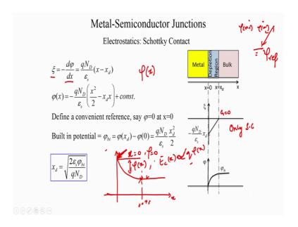
So, for example, an equally valid reference is you know choosing the potential in the bulk as a reference. So, if this is the band bending and say that is x equal to x d. We could say that that is the reference potential that is phi equal to 0; no problem. As long as you apply the correct boundary conditions it is absolutely no problem as to what you take as your reference potential.
