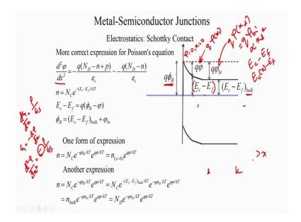
So, the way this comes about is let us say d E by d x is equal to rho by epsilon s where rho is the charge concentration. Now clearly, since E is equal to minus d phi by d x you have d square phi by d x square is equal to minus rho by epsilon s. So, you need to have a minus sign in place that.
