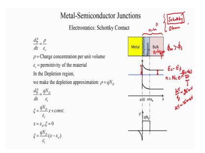
And we already saw that the Fermi levels will align, the semiconductor will give electrons to the metal because your phi m is greater than phi s and this is an n-type semiconductor. So, the electrons will move into the metal, and the conduction band will bend away from the Fermi levels, and this will be the band bending diagram.
