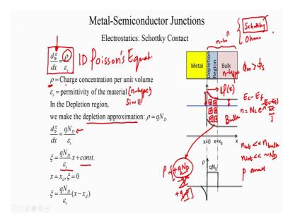
So, the potential is varying with distance so, the potential is a function of x. And therefore, there is an electric field so, whenever you see a bent band it means that there is an electric field in that region. So, very far from the junction, you know there is once you cross this point there is no more band bending ok.
