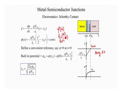
So, if you can find the variation of the potential in the semiconductor with x you have essentially found the nature of the variation of the conduction band bending with x, the nature of the variation of the valence band bending with x etcetera. So, how do we calculate the potential variation? Now the electric field is nothing, but minus d phi by d x ok.
