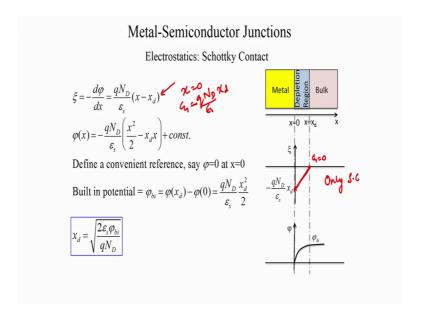
So, if you have to plot this electric field so, in the semiconductor, so again it is this plot is there only in the semiconductor. So, we are looking at only the semiconductor at x equal to 0. So, if you were to take this expression here at x equal to 0, the electric field is q N D by epsilon s x d with a negative sign.
