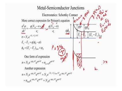
So, what we are going to do? Is we are going to perform the study in a region of the depletion in the depletion region, but closer to the bulk as compared to the interface ok. So, we need a more accurate Poisson's equation and we say that although we could retain p we say that p is negligible, but there is no need because we have no information.
