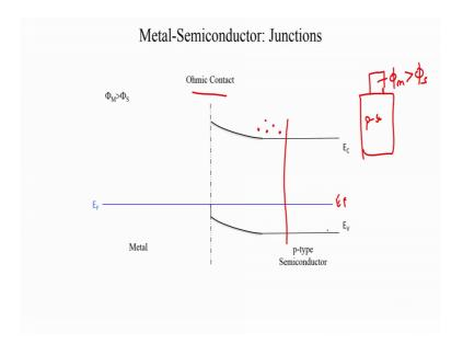
So, the band bending would look like this ok. So, you have your E f, the E f is aligned but since the semiconductor gave electrons to the metal, the conduction band edge moves away from the Fermi level and the valence band edge follows.
