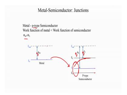
Finally, we will take the fourth of the cases ok. It is a metal P type semiconductor junction but phi M is now less than phi S which means that you have your P type semiconductor ok.
