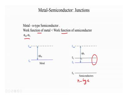
So, let us say we again have a metal semiconductor junction. And let us say the semiconductors still an n-type semiconductor, but this time we will let the work function of the metal will be less than the work function of the semiconductor which means phi M is less than phi S, ok.
