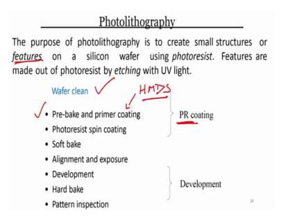
All right; that means you have to coat the photoresist, so, before photoresist the primer coating, is sometimes you will see a word called HMDS. HMDS this is your primer, all right so, for improving the adhesion of photoresist onto the oxidize silicon substrate, or onto the metal over the oxidized silicon substrate, sometimes we use a primer called HMDS all right. So, first step is your pre-bake and primer coating, second is photoresist spinning. So, this first step this is second step.
