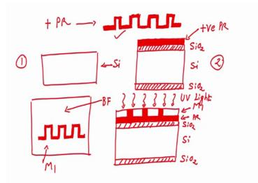
So, next step would be we will load this mask. So, I will draw the wafer once again, then we have oxide, then we have photoresist, right and then we will we have done soft baking already, we have completed soft baking. So, what is the next step next step is we have to load the mask, load the mask where, load the mask on this wafer.
