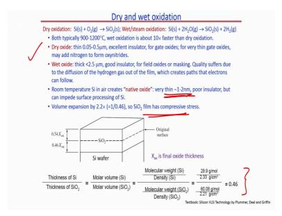
So, let us go to the next slide or the next part of this particular slide and that is that both of these oxidations are done at 900 to 1200 degree centigrade both of these oxidation are carried out at 900 to 1200 degree centigrade, where wet oxidation is about 10 times faster than dry oxidation.
