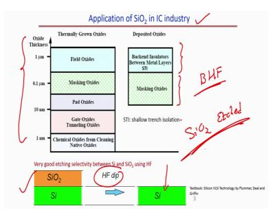
Now, let us move to the next one. So, very good etching selectivity between Si and SiO 2 using HF. If I have a silicon dioxide on silicon which is this one and if I dip it in HF, I told you we can use buffer hydrofluoric acid or we can use hydrofluoric acid, if we dip it what we
