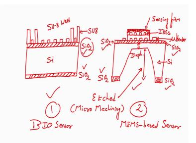
Today, we are learning the thermal oxidation process. So, if you come back on the screen and if you focus the thing that. We have seen until now I think that we have seen until now are 2 devices; one is an interdigitated electrodes in an SU-8 well and in both the cases what we have seen, there is silicon substrate and there is silicon dioxide. This is SU-8. This is first device that we have seen, number 1.
