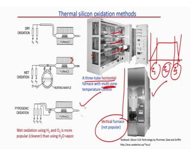
Now, what next we have to see? We have to see the thermal oxidation methods. First, is your dry oxidation, second is your wet oxidation, third one is your pyrogenic oxidation. In all the cases, what we see one thing common is, there is a furnace, there is a horizontal tube furnace you see. The tube is in horizontal direction that is why it is called horizontal tube furnace. If tube is in vertical direction, vertical tube furnace; tube is in horizontal direction, horizontal tube furnace.
