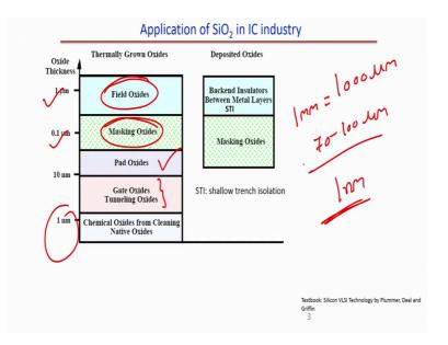
Now, what I am saying is human hair is about 70 to 100 micrometers, you see and what we are talking about we are talking about 1 nanometer. So, it is extremely thin. For this, we can use as a chemical oxides from cleaning native oxide. So, if this is the case if you want to remove the clean the native oxides the chemical oxides from the native oxides we can have thickness of about 1 nanometer.
