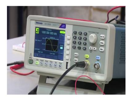
Yeah ok, so now, you can see it is already 500 millivolts, or we can say 0.5 volts at 1 kilo hertz frequency applied to the non-inverting amplifier of the non-inverting operation amplifier.
