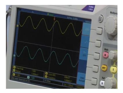
So, see guys try to understand oscilloscope, right. In case out of any reason you are not so familiar or you feel that you know how to adjust the things, just press auto scale button if there is one on your oscilloscope. It will auto scale it and it will be very easy for you to understand.
