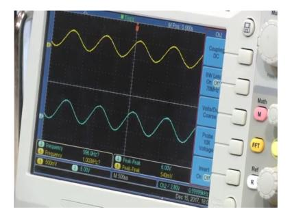
You can see blue color thing, right? 6.2 volts at the output, and the input is yellow one peak to peak 540 millivolts; that means, still the output has not been clipped so, 0.5 is ok, right, this depends this depends on your gain. So, do not forget, if you set a gain extremely high, then even 0.5 will be your voltage range.
