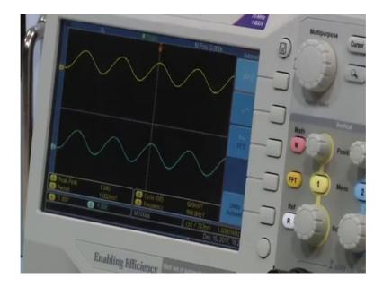
So, output will follow the input voltage follower, output will follow the input without any amplification, without an amplification.
