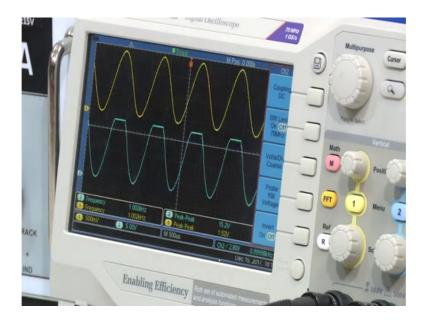
And now we can see there is a clipping, clipping occurring, right. Because the output peak to peak you see is around 15 volts, 15 volts very close to our bias voltage, suddenly, we will see the clipping; that means, that from this kind of experiments, we can easily find what is the input voltage range, what is the output voltage range?
