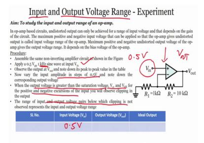
Here we will apply 0.5 volts peak-to-peak frequency, we can have 1 kilohertz, right. And we will keep on increasing this in a step size, see one once you apply 0.5 volts we will see what is the output voltage V out, right. Then we will apply another we 0.5 to 0.5 that will be 1. So now, we vary the input amplitudes in steps of 0.5 volts and note down the corresponding output voltage; that means, initially 0.5, then 1 then 1.5 then 2 then 2.5.
