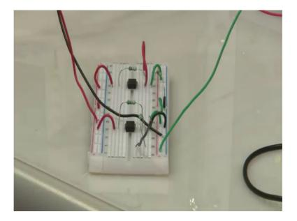
So, if you see the breadboard, then the breadboard we have already connected the noninverting amplifier, we have not given the input signal to the non-inverting amplifier yet, but the circuit; that is, where I am pointing my finger, right, this particular circuit or this one here, right. This is the non-inverting amplifier, now do not get confused is not really different, it is same thing that we have seen on the screen exactly same thing, right?
