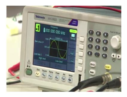
1 volt if you see high it is 1 volt is applied, right, what is the frequency? 1 kilohertz is the frequency voltage is 1 volt, right. Voltage is 1 volt, and frequency is 1 kilohertz, this is the input signal.
