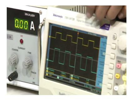
So, if you see it is around 11 volts 11 volts peak-to-peak when we apply 11.2 to 12 volts peak-to-peak, right blue one. And the input voltage is 1.04 volt; that means, that it is amplified the signal is amplified.
