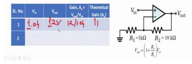
What is V out by V in 12 divide by 1.04, that is your gain. So, easy theoretical gain R 2 by R 1 into 1 plus R 2 by R 1. So, what is that? 1 plus R 2 by R 1, 1 plus 10 by 1, right? 1 plus 1 by 1 is 1 plus 10 or 11.
