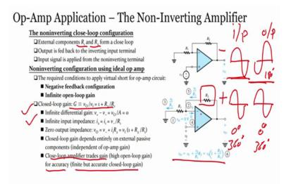
This is output, alright, then in case of non-in in case of inverting amplifier, I am writing just minus as inverting amplifier, signal if I apply here, output would be opposite, right, 180-degree opposite.
