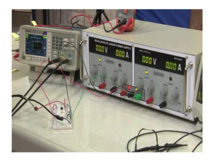
Here we have plus 15 minus 15. So, we can first connect it here, and then we can apply the DC power supply, first we can connect and then if you apply, alright. So, what he is, right now performing is he is connecting the bias voltage is plus 15, minus 15 to the inverting amplifier using op amp, alright? And we already have grounded.
