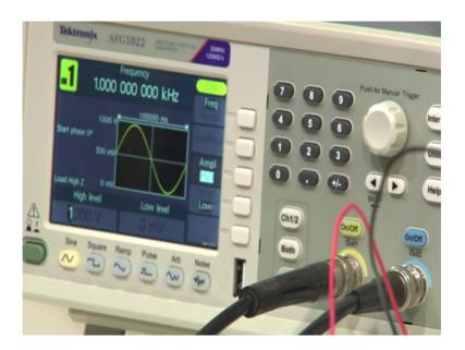
Let me just yes, so, if you see here, we are applying one kilohertz frequency. What is the voltage? We are talking about peak to peak voltage, right. So, you see what is the peak to peak voltage, peak to peak voltage is one volts, right, you see there is a 1 volt. Now this signal we have to apply to the inverting terminal. So, when you see that you will see the probe, which is holding in his hand. So, you see this probe that is holding here, look at this probe, right.
