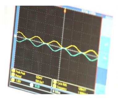
What is the new value? You use again there is a phase shift the output voltage now is from one volts, it is about 5 volts. See peak to peak is 10, but the voltage that you can see at the output is nothing but 5 volts, alright. So, or you can say 520 millivolts. So, applying 500 millivolts at the input, sorry, 500 millivolts at the input what is the output that we have to see, right?
