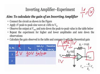
So, how to perform or how to calculate the gain of an inverting amplifier. Now given that you are have, R 1 equals to 1 kilo ohm this one, right. Feedback resistor R f equals to 10 kilo ohm, what will be the gain of this particular amplifier? So, first thing we have to understand what is the circuit, if you see closely, right what actually the circuit is? The circuit is that the input signal, the input signal is given to inverting terminal right; that means, it is an inverting amplifier.
