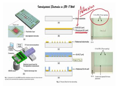
Then we came to this particular slide and then we have seen how you can create or fabricate int or interdigitated electrodes. An interdigitated electrodes right with metal that is chrome and gold; I said that chrome is used to improve the adhesion, a, d, h, e, s, i, o, n, adhesion of gold of gold right.
