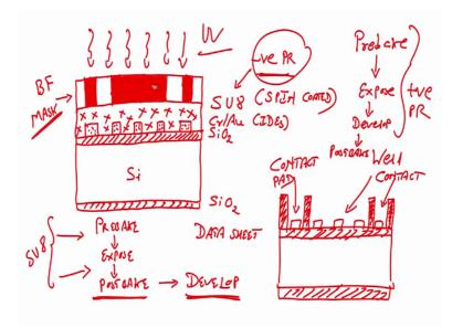
See pre-bake positive we are talking about positive then you have to expose then you have to develop then you have to post bake right pre-bake expose develop post bake this is the case of positive photoresist right.
