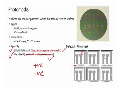
Now, this is not always true that bright field mask is used with negative for this or dark field mask is used with for positive photoresist. We have just seen an example where bright field mask can also be used with positive photoresist. Bright field mask can also be used with negative photoresist. So, so I believe that this sentence does not hold true in all the cases, but the masks are of two types that is completely correct. Bright field mask and dark field mask alright.
