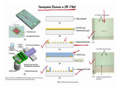
Patterned electrodes we quote, we spin coat SU 8. You can see here we have spin coated SU 8. On the spin coated SU 8, what we will do? We will pre-bake it. Then we will load the mask, we will expose the SU 8 right and then we will do post baking. Then we will develop and then when we developed, we get this particular wafer, this particular glass. Glass with interdigitated electrode in the SU 8 well you got it.
