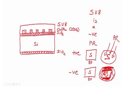
I will which wafer which already has the interdigitated electrodes. So, I can directly draw oxidized silicon wafer on which I have chrome gold. Right chrome gold has interdigitated electrodes. On this on this I will spin coat SU 8. Alright SU 8 is a negative photo resist. Until now what we have seen? Positive photo resist right positive photoresist, what happens? If I have a mask then my wafer would have same pattern. In negative this is my bright field mask.
