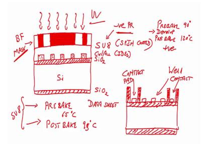
So, when you have SU 8 as a negative photoresist, you how can you make the well? Right your idea is your final idea is that you should have a substrate you should have a substrate right. Let me remove this you have a substrate with interdigitated electrodes and then you have SU 8 well. This is what you want this is what you want right this is the well. This is for the contact right this is also for the contact pair contact right.
