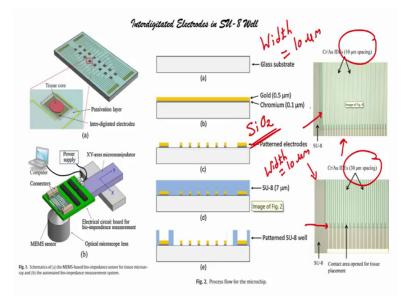
Alright, what we see is there are interdigitated electrodes with spacing. So, the width w i d t h width is 10 micrometers and spacing is 10 micrometers.
