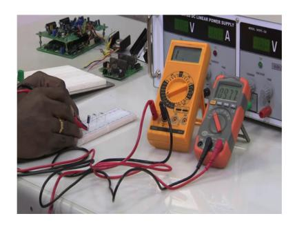
So, you can see the first thing that he is doing is he is using the resistance, right. You see resistance he has kept around 20 kilo ohm. So, you can you can start at any value if you do not know the value. And you can keep on increasing the this probe to higher values. So, the first thing he has tried 20 kilo ok, let us see now.
