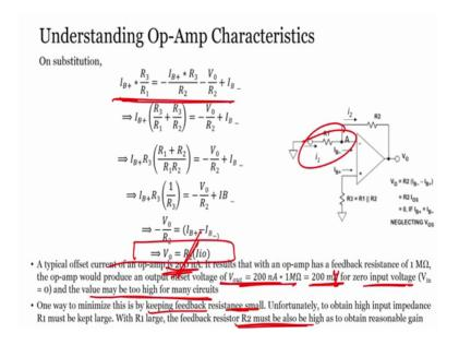
Now if you substitute on substituting the values we will have I B plus into R 3 by R 1 equals to minus of I B plus into R 3 by R 2 minus V o by R 2 plus I B minus. So, if I solve this equation further what I will have V o will be equal to R 2 into I I o right.
