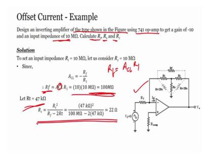
Now, let us take an example, let us take an example design an inverting amplifier of the type shown in figure using 741 to get a gain of minus 10 and input impedance of 10 mega ohms right also calculate R t R s and R 1 this are the this are this is the problem. So, let us find the solution since what we said gain is nothing, but minus R f by R 1 we have R f is equal to gain into R 1 this is c l should be subscript. So, we can say R f is nothing, but R f is nothing, but gain into R 1.
