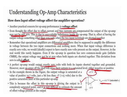
Now, let us see another point another point that is we have to understand the effect of input offset voltage on the amplifier operation, we will see now effect of input offset voltage on the amplifier operation. So, what is the input offset voltage, we already know right another practical concern Op Amp is voltage offset even though the effect due to the offset current and bias current are compensated.
