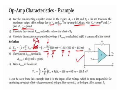
So, let us see an example. So, Op Amp characteristic we are looking at as an example first is for the non inverting amplifier shown in figure this one, R 1 is one kilo ohm R f equals to ten kilo ohm calculate the maximum output offset voltage due to V o s in I B. The Op Amp is 1 m seven 1 m 307 where V o s is ten millivolts and I B 300 nano ampere I I o V is 50 nano ampere right. So, the first thing is we have to calculate the maximum offset voltage.
