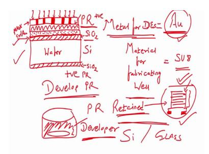
So, after positive photoresist once I load the mask once I load the mask if I do the UV exposure with UV light then what I will get after this one after UV light. So, after spin coating loading, loading mask the performing UV exposure I have to develop develop my photoresist, develop my photoresist, all right.
