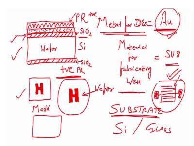
And if I use positive photoresist, if I use positive photoresist, then I on my wafer on my wafer I can very bad drawing once again ok, on my wafer I will retain this similar pattern, I will retain similar pattern which is which is the same like my mask, which is similar to my mask, all right.
