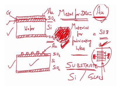
Next step is we have to, we have to form the inter digitated electrodes right. So, what we want is this is a cross sectional right do not do not get confused when I am drawing cross section, this is your silicon dioxide this is your silicon dioxide right SiO 2, SiO 2, Si this is your chrome gold or I will just say gold. Make it easy ok. It is always a chrome gold, this is what we want from this wafer, from this wafer, all right.
