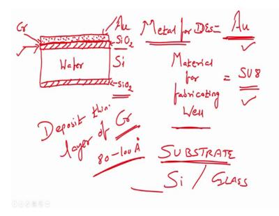
Then the adhesion would be better, then the adhesion would be better, all right this much easy, this much is easy, right. What what we have said that if I directly deposit gold on the substrate it has a poor adhesion, but if I use a thin layer of chromium and then deposit gold the adhesion improves adhesion improves, right. So, that is a next step. Why? Because we wanted metal for interdigital electrodes right which is your gold, which is your gold, right.
