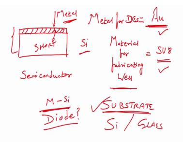
So, metal, let us write down here metal. Metal is what? Gold right, then it will we need material, material for fabricating fabricating well this material is SU-8, all right. What is this? First one is unique wire metal metal for inter digitated electrodes right which is our gold, metal for then material for fabricating well which is the SU-8. So, these two things we require, we got it.
