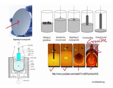
This is a very at very high temperature very high temperature. So, that this silic polysilicon is melted, polysilicon is melted, once it is completely melted then only we introduce you this seed crystal once it is melted then you introduce seed crystal ok, all right. So, this is how the boule is fabricated nice.
