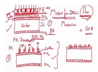
Now, what you have? You have, you have photoresist and photoresist is saving your photoresist is this one on the top photoresist, this one is photoresist, this is photoresist, on the top this one is photoresist, this one is photoresist, on the bottom, on the bottom this 5 blocks that you see these are nothing, but chrome gold right, this is chrome gold, this is chrome gold correct.
