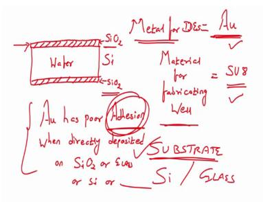
But if the gold has poor adhesion poor adhesion when directly deposited when we directly deposit direct, when directly deposited on SiO 2 or glass or silicon or any other substrate what is that; Au has poor adhesion. Adhesion is nothing, but sticking property, all right, if it does not stick properly then we cannot use it further. So, it has a poor adhesion, it has a poor adhesion.
