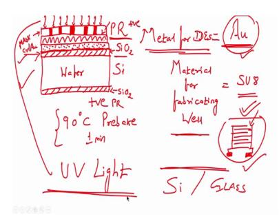
After spin coating photoresist you have to pre bake it at 90 degree centigrade, pre bake at 90 degree centigrade for 1 minute, all right pre bake at 90 degree centigrade for 1 minute. After pre baking for 90 degree centigrade for 1 minute, we will we will keep the mask we will keep the mask on the positive photoresist on this wafer the mask has the pattern right.
