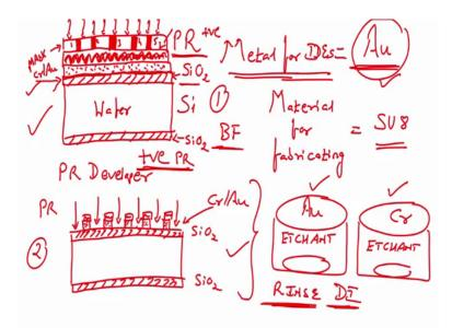
So, what I will do is I will first etch my gold first I will etch my gold by dipping my this particular wafer into the gold etchant Au etchant E T C H A N T, all right. After that I will take the wafer and and use DI water DI water right to rinse it to rinse it, r i n s e, rinse, right I will use DI water and I will rinse the wafer then I will dip this wafer in the chrome etchant e t c h a n t, all right.
