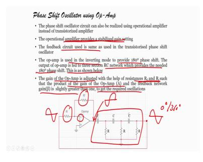
So, if I want to design a phase shift oscillator using an operational amplifier if I want to design a phase shift oscillator using an operational amplifier, how will I design the phase shift oscillator can also be realized using op amp instead of transistorized amplifier op amp provides a stabilized gain setting the feedback circuit used is same right you can see here if I use transistor base amplifier then in also.
