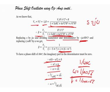
Now, as we know that V o equals to V f is I 3 into R. So, if I substitute the value, then we have beta equals to n beta equals to V o by V i, I will have this value. So, replacing s by j omega because we have considered s equals to j omega right here.
