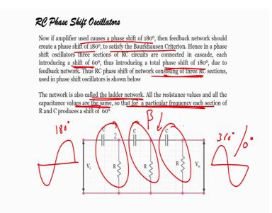
This one is my beta. So, if I apply output voltage which is 180 degree of phase shift or out of phase with input then my feedback to the input will again be a 0 degree because 180 plus 180, this is 60 from here, 60 from here 60 from here.
