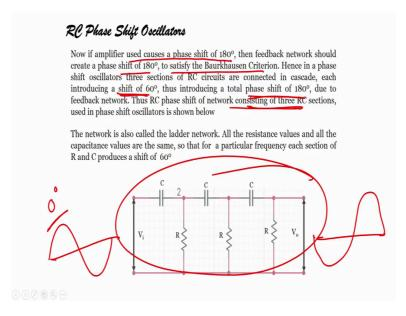
Hence, in a phase shift oscillator 3 R sections of RC circuits are connected in cascade each introducing a phase shift of 60 degree each introducing a phase shift of C 60 degree does introducing a total phase shift of 180 degree this is what we have discussed right thus RC phase network consists of 3 RC sections as shown below which is shown right over here.
