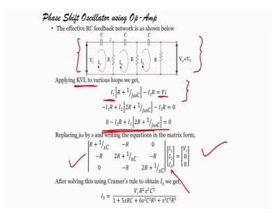
So, the effective RC feedback network is shown in figure here right. So, this is V I, this is V o equals to V f. So, applying k V L to various loop what we have what we will have is I 1 into R plus 1 by j omega c minus I 2 R equals to V i right now if I solve this thing if I solve this equation, what will I have; what will I have this in particular equation.
