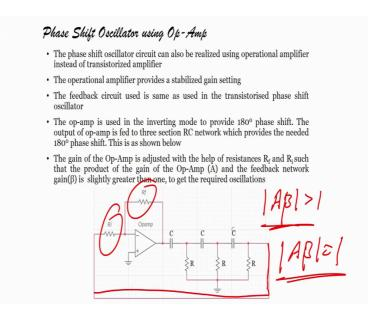
Once the oscillations are is by a beta should be equal to one right. So, this you can change by changing the value of RF and R I, this you can change by changing the value of RF and R I, this feedback here it is connected here its connected here through the from output to the input from output of the beta that is feedback network to the input of the oscillator.
