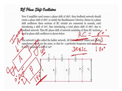
So, if I want one RC is 60 degree. So, if I have a amplifier that is my inverting amplifier inverting amplifier, right if I apply a signal, then my output would be 180 degree out of phase, this is 0, this is 180 degree; that means, my feedback should produce another 180 degree phase shift. So, that my feedback signal will also be 0 degree, correct, this we have seen.
