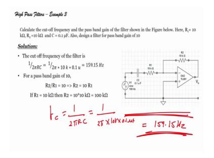
So, let us see one more example calculate cutoff frequency and the pass band gain of filter shown in the figure. So, suppose you are given this figure right. So, what is this figure this is nothing, but my this is nothing, but my high pass active filter right high pass active filter now what I had to find I had to find the I had to find the cutoff frequency; that means, I had to find f c right f c is one upon 2 pi R C.
