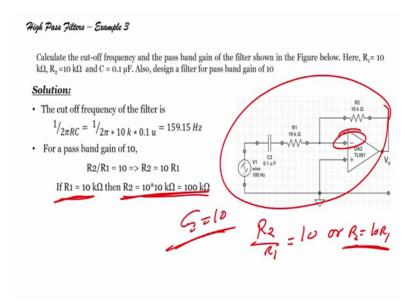
So, here it will be R 2 by R 1 equals to 10, right why because inverting amplifier it is a inverting amplifier. So, R 2 by R 1 equals to 10 or R 2 would be equal to 10 times R 1 right.
