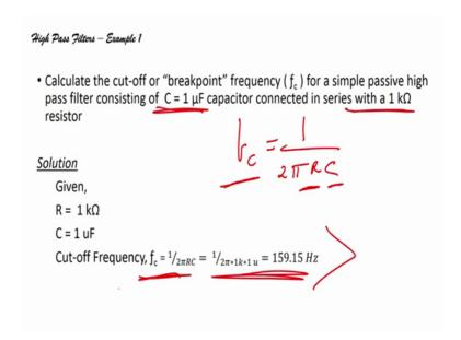
So, if I take an example if I take an example. So, if calculate the cutoff frequency or break point frequency f c; so, f c formula we can directly write one upon 2 pi R c or one by 2 pi R C for a simple passive; passive high pass filter consisting of capacitor c equals to one micro farad. So and connected in series with one kilo ohm resistor I have value of R I have value of C. So, I can find the value of f c, I can find value of f c, right.
