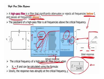
A high pass filter is a filter that significantly attenuates or rejects all the frequencies below f c below f c and pass passes all frequencies above f c. So, what is that filter a filter is that all the frequencies below f c it will reject while above f c it will it will pass.
