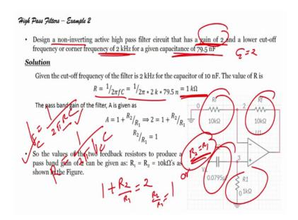
Let us say another example design. Now you see you have to design; design a non inventory active high pass filter such that gain equals to 2 low lower cutoff frequency or corner frequency is 2 kilowatts and capacitance of 79.5 nano-farad, alright these 3 things are there
