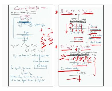
That is in this case my V G S is greater than 0 volt, V G S is greater than 0 volt; see if my V G S is greater than 0 volt, let us assume it is plus 1 volt. You can see here plus at gate terminal; you have substrate, you have substrate which is connected to the ground or it connected to the ground and also internally the connected to the source that we know. So, here if I have gate which is positive compared to source.
