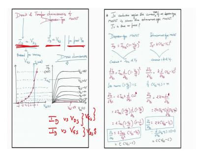
What I am saying is if I know the plot I D versus V D S, how it looks like. It is for different value of V G S; for V G S different values. Then it is extremely easy to plot I D versus V G S for same V D S; for same V D S, very easy is not it; extremely easy.
