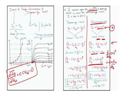
For the depletion MOSFET is C V G S minus C. This is my equation. For what? Depletion type MOSFET and the 2 in conduction region, the great of change of current.
