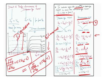
So, I have value d by d I D by d V G S equals to C times V G S minus C. This is what I have derived; this is what I have derived. This is for Enhancement type; Enhancement type. This is for Depletion type; Depletion type MOSFET.
