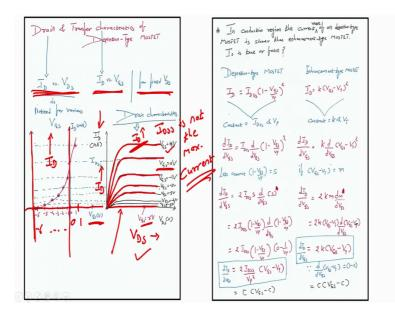
So, in this case if I want to draw a drain transfer characteristics, drain and transfer characteristics for depletion type MOSFET. How can I draw it? Now you see here, see this case here you see at V G S equals to 0 volt I already have on increasing V D S, on increasing V D S, I will see increase in I D. You see here let us consider V G S equals to 0 volt; that means, we have to consider this line and you see here there is a current already flowing right in case when V G S is 0 volt.
