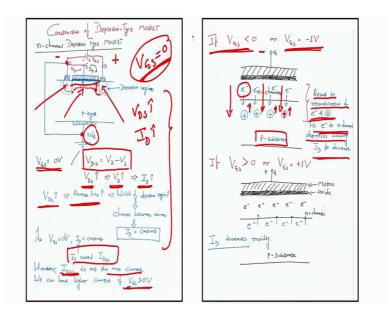
So, you see this slide, we will see or you can see what is here. This particular figure if you see, there is a substrate which is SS slash B; this is internally connected to the source
