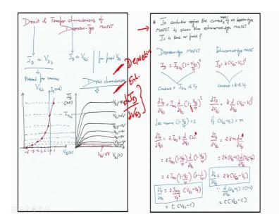
Here, the problem is in the conduction region; in the conduction region the rate of current, the current rate of an depletion type MOSFET; the current rate of an Depletion type MOSFET is slower than Enhancement type MOSFET. What is written? The sentence written is let us read it together in the conduction region, the current rate of an depletion or of a depletion type MOSFET is slower than the current rate in enhancement type MOSFET, is this statement true or false that is a question.
