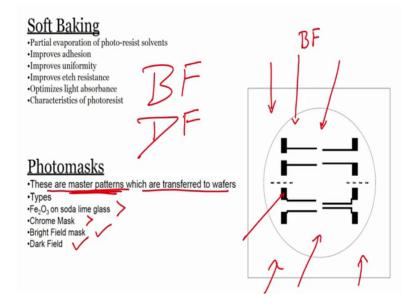
So, these are master patterns which are transferred to the wafers right, whatever there is of the mask we can transfer it onto the wafer that is why these are called master patterns, master patterns right.
