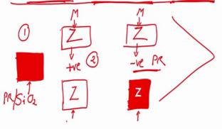
So, photoresist is nothing, but a polymer and it is a solid organic material it is nothing, but a solid organic material. The advantage of this is it can be used to transfer the design pattern to the wafer surface. We will see an example. So, you understand how it is used.
