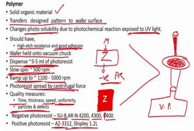
So, next step is after this after this we can what we should do we should. So, how we can coat this photoresistor is a question, how we can coat the photoresist. So, you guys are understand this particular thing right. So, I am removing it. So, that you can see what is written I am removing this schematic. Now you can see.
