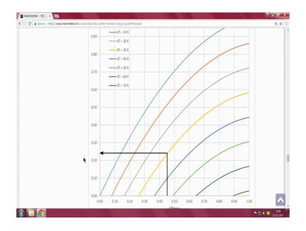
Heat pumped versus current. So, you see now Q c by Q max you know is typically around 0.25.
