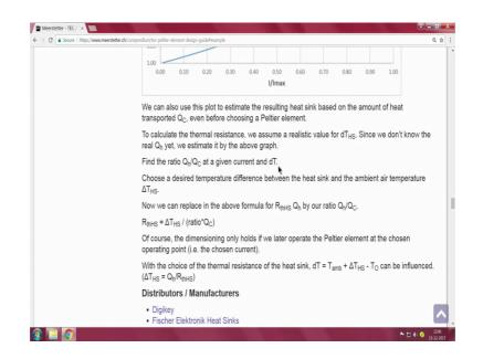
We can use this plot to estimate resulting heat sink based on the amount of heat transported even before choosing a Peltier element. To calculate thermal resistance we assume a realistic value of delta T at the heat sink. Since we do not know the real Qh at to be estimate by the above graph find the ratio choose a desired temperature difference and so on and then finally, we come to this fan thing.
