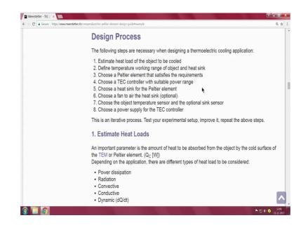
First of all the most important point here is to estimate a load without the load estimation. First of all estimate the heat load of the object to be cooled then define temperature working range of object and heat sink.
