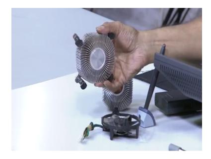
However if we do break it open, chances are it has a high conductivity copper core inside. The advantage of it is to make this heat sink effective that is there is a the think about fin
