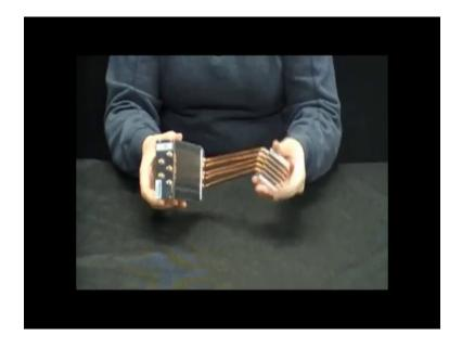
(Refer Time: 20:25) experience with designing and manufacturing heat pipes and heat pipe assemblies heat pipes are the best way to transfer heat spread heat or increased heat sink fit efficiency. His custom avid heat pipe assembly this assembly can dissipate up to 150 watts heat pipe assemblies have three zones that contribute to the heat transfer ability the first zone of the heat pipe the evaporator is where the heat absorbed from the device evaporates local liquid into a vapor.
