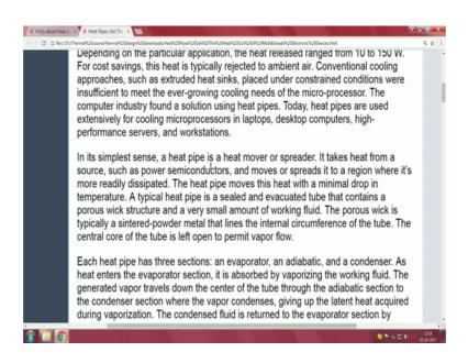
In its simplest a heat pipe is a heat mover or spreader takes heat from a source such as power conductors and moves it to a region where it is more readily dissipated. Heat pipe moves this heat with a minimal drop in temperature; typical heat pipe is a sealed and evacuated tube that contains a porous wick structure and a very small amount of working fluid.
