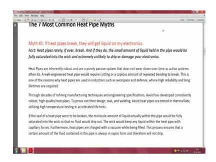
Now, myths I think you should read it yourself; it is not liquid cooling it does not need type of pressure tight what you call design. And it is generally being under vacuum and the moment any leakage comes no liquid will ever come out and likely to short circuit your device as compare to water cooling or other things ok. The miniscule amount of liquid actually within the pipe would be fully saturated into the wicks or now fluid will drop out.
