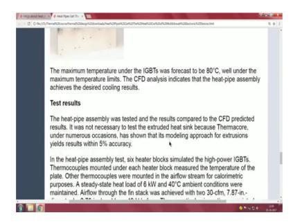
Test results heat pipe assembly was tested compared to the CFD predicted; six heater blocks simulated the high power IGBTs; thermocouples mounted and so on; acoustical noise is a thing.
