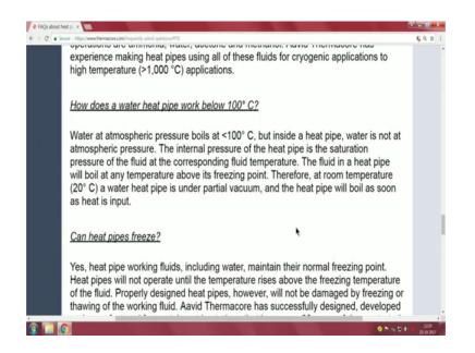
So, we have working fluid helium and nitrogen for cryogenics to liquid like sodium and potassium metals for high temperature heat dissipation; more common heat pipes used ammonia, water, acetone and methanpl. You can make it yourself you go to YouTube I will show you one or two pictures of those things.
