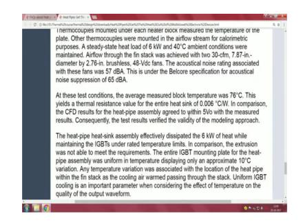
At this stat condition the average measure block temperature or 70 to 76 degrees; this yields a thermal resistance value of the entire heat sink of 0.006 degree centigrade per watt.
