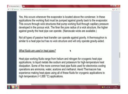
But then remember some of the game places even first liquid cooling is used. And we come to important thing can they work against to gravity are it has to be horizontal. The pictures they have shown there is shown horizontal; in these applications working fluid must be pumped against gravity back to the evaporator. This occurs through wick structures and pump working fluid through capillary pressure; finer the pore radius of a wick structure the higher against gravity nanoscale.
