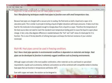
Next it has to be very hot for heat pipes to work; that is another thing which is true in the case of actual simple convective heat sinks, but in the case of what you call heat pipes we have a control of it. The temperature of the heat source does not need to reach the standard room temperature boiling point to cause the liquid to change. In fact, a few difference is needed between hot and areas of a heat pipe to make it function one of the advantages.
