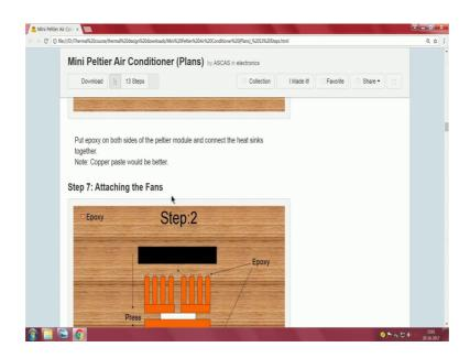
Connect the heat sinks together copper paste you see here very nicely very nicely very very properly he has given know if you can get a loaded copper paste like thing. It will
