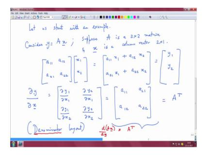
So, let us just start with an example. So, consider A times x. So, y is some A times x suppose A is a 2 by 2 matrix and x is a column vector and this is say suppose 2 by 1 right.
