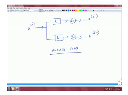
This goes through filters 1 and h, then there is down sampling by 2 and you have a j minus 1 here and you have b j minus 1 here. This is basically like the analysis, analysis stage of a filter bank. We have done nothing except that we have sort of interpreted the wavelet decomposition through filtering the coefficients from s k 1 j through appropriate filters ok. Now we can think about it in a similar way for the reconstruction procedure.
