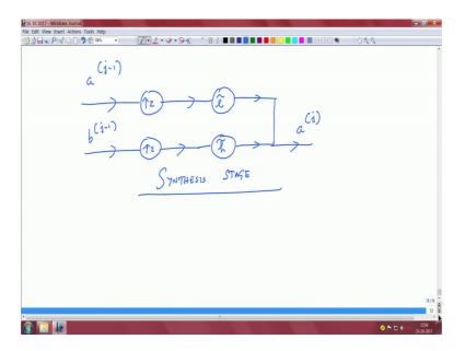
So, we can think of a j minus 1 being sampled and then going through this filter 1 tilde and we have b j minus 1 being up sampled going through this filter, h tilde and then combining them to get to give you a j right and this is basically the synthesis stage ok.
