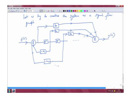
So, let us try to realize the system as a signal flow graph now how do we get this graph. Now, we have various tab delays, now we have a forcing function f of n. At this point it is scaled by b 0 and gets to the output, then f of n going through this delays f of n minus 1, f of n minus 1 is scaled by b 1 and then gets to the output so on and so forth.
