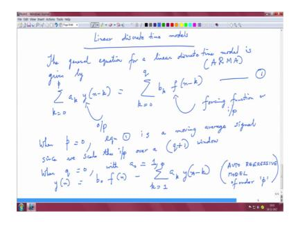
So, the general equation for a linear discrete time model is given by summation a k y of n minus k, k going from 0 to p equals summation b k f of n minus k, k equals 0 to q. So, this f is basically the input or the forcing function, and this is the output, y is the output which self expresses itself with various delays, it self expresses itself with various delays.
