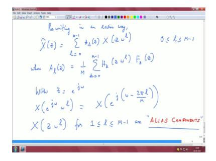
Rewriting in an easier way X hat of Z is summa l equals 0 to M minus 1, A l of Z times X Z omega power l, where A l of Z equals 1 upon M summa k equals 0 to M minus 1 H k of Z omega power l F k of Z for all the M components, ok.
