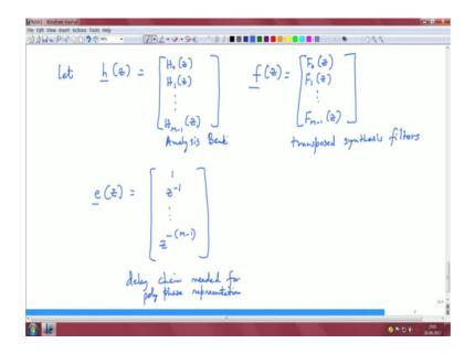
Let h of Z be a column vector comprising of the analysis bank, this is H naught of Z, H 1 of Z dot dot dot H M minus 1 of c this is a column vector similarly we have f of Z is a stack of the transposed synthesis filters.
