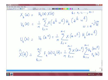
So, we start with the usual analysis that we are comfortable X k of Z is H k of Z times X of Z and of course, this is k equals 0 1 dot dot dot till M minus 1 right. If you recall for a 2 channel filter bank we had just k equals 0 and 1 just two components here we have M components 0 to M minus 1. So, therefore, X k of Z is this for k equals 0 to M minus 1.
