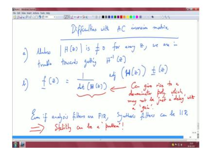
Unless the magnitude of H of Z is not equal to 0 for every Z we are in trouble towards getting H inverse of Z, right. I mean because if you think of realizing H of Z as magnitude of H of Z times some E power j phase and if you have inverted you are having a 1 over the magnitude of H of Z in the denominator right and that should not be 0.
