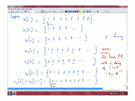
So, let us take for granted that x of n is suppose x of n is a ramp maybe I just take about 8 values 1 2 3 4 5 6 7 8 dot dot dot, ok. Now, v naught of n is the down sample signal right. So, basically we have only the odd components 1 3 5 7 so on because we are considering only the alternative samples here alternate samples.
