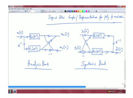
So, let us look at the signal flow graphs for this for realizing these filters for a polyphase realization. So, we will start with analysis bank. So, we have x of n this goes through the filter E naught of Z square, then I have a delay element this is filtered through the filter E 1 of Z square.
